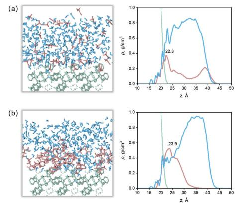
Fig. 6 Configurations of surface–solvent interfaces (left) and mass density profile along the normal to the crystal faces (right) for the (110) face from the MD equilibrium. (a)  $Ca(Min)_2-MeCN-H_2O$  interfaces. (b)  $Ca(Min)_2-DEF-H_2O$  interfaces. Surface is in green, organic solvent is in red, and water is in blue.
