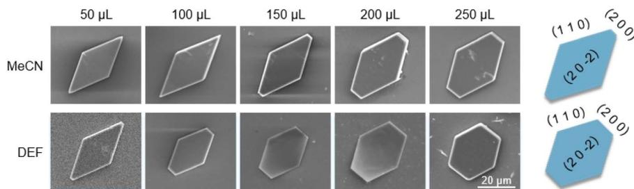
Fig. 4 Experimental morphology of Ca(Min)<sub>2</sub> after adding 50–250 μL organic solvents (left five SEM photos) and simulated morphology in 25 vol% organic–water solvent (right pictures, corresponding to a little higher than 250 μL in experiment).
