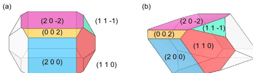
Fig. 3 Morphology (front (a) and 45° side (b) views) of  $\text{Ca}(\text{Min})_2$  predicted in vacuum.
