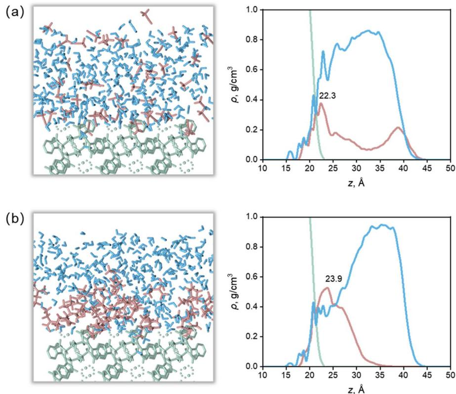
Fig. 6 Configurations of surface-solvent interfaces (left) and mass density profile along the normal to the crystal faces (right) for the (1 1 0) face from the MD equilibrium. (a) Ca(Min)<sub>2</sub>-MeCN-H<sub>2</sub>O interfaces. (b) Ca(Min)<sub>2</sub>-DEF-H<sub>2</sub>O interfaces. Surface is in green, organic solvent is in red, and water is in blue.
