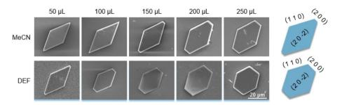
Fig. 4 Experimental morphology of Ca(Min)<sub>2</sub> after adding 50-250 µL organic solvents (left five SEM photos) and simulated morphology in 25 vol% organic-water solvent (right pictures, corresponding to a little higher than 250 μL in experiment).
