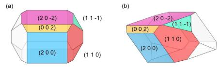
Fig. 3 Morphology (front (a) and 45° side (b) views) of Ca(Min)<sub>2</sub> predicted in vacuum.
