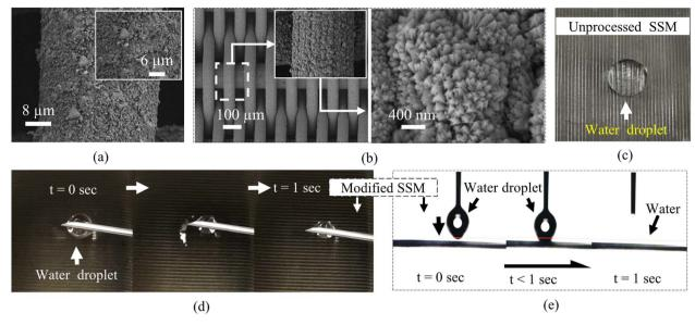
Fig. 6 SEM and WCA measurements of the SSMs (a) SEM of the hydrothermally treated for 12 hours SSM with TiN300 film, (b) SEM of the hydrothermally treated for 8 hours SSM with TiN300 film, (c) a water droplet on the unprocessed SSM, (d and e) time sequence of a water droplet spreading on the modified SSM.
