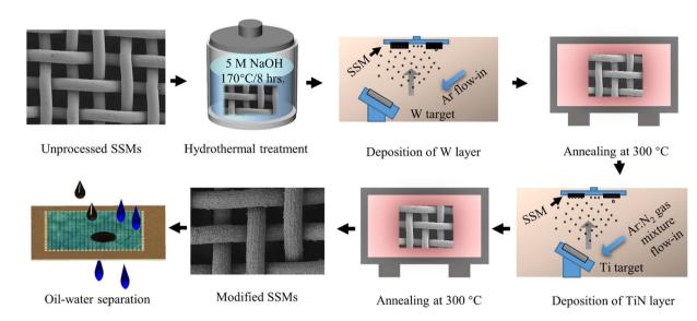
Fig. 1 Schematic diagram of the fabrication procedure of the proposed surfaces.
