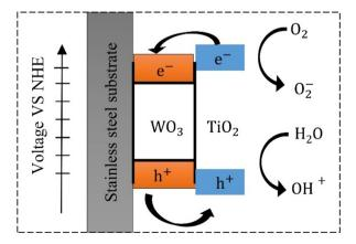
5 Schematic illustration of the photo-induced hydrophilicity of the thin TiN300 film.
