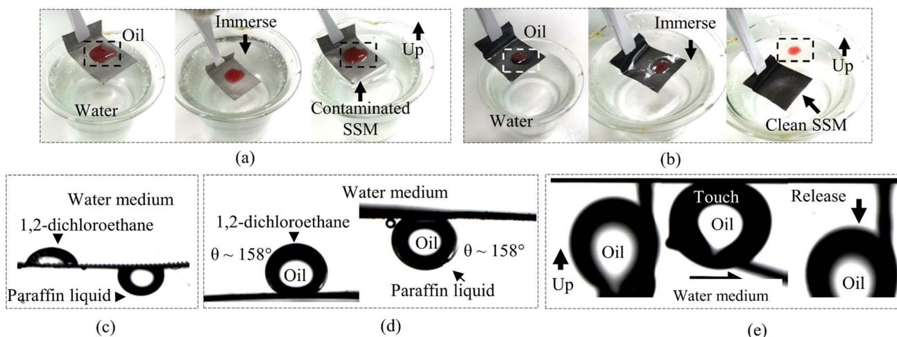
Fig. 7 Oil contamination tests (a) paraffin liquid on the as-received SSM, (b) paraffin liquid on the modified SSMs (c) UOCA on the unprocessed SSM, (d) UOCA on the modified SSMs (e) paraffin liquid adhesion test on the modified SSMs.
