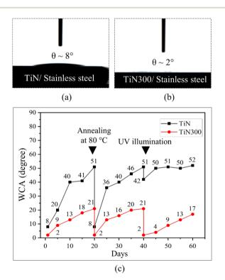
Fig. 3 WCA measurements on TiN and TiN300. (a) WCA on TiN on day one, (b) WCA on TiN300 on day one, and (c) change of WCAs on TiN and TiN300 from day one to day 60 under the effect of dirt contamination, post-annealing, and UV light illumination.
