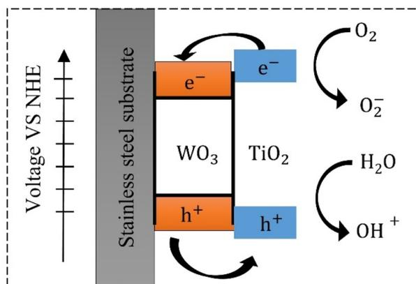
Fig. 5 Schematic illustration of the photo-induced superhydrophilicity of the thin TiN300 film.
