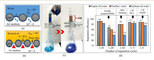
Fig. 9 Oil-water separation mechanism and efficiency (a and b) oil-water separation mechanism using a superhydrophilic mesh, (c) oil-water separation process using the modified SSMs, and (d) oil-water separation efficiency.
