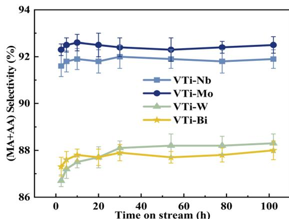
Fig. 11 Durability of (MA + AA) selectivity test over the metal cation-doped VPO catalysts in TOS of 100 h.
