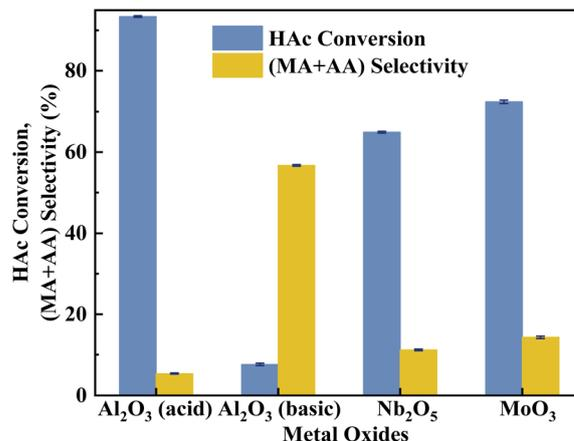
Fig. 9 Catalyst performance of metal oxides. The reaction temperature and carrier flow rate was  $360 \text{ }^\circ\text{C}$  and  $50 \text{ mL min}^{-1}$  ( $3.0 \text{ vol}\% \text{ O}_2$  in  $\text{N}_2$ ), respectively. The liquid feed was a HAC-FA mixture (2.5/1,  $n/n$ ), with a LHSV of  $1.33 \text{ mL h}^{-1} \text{ g}_{\text{cat}}^{-1}$ .
