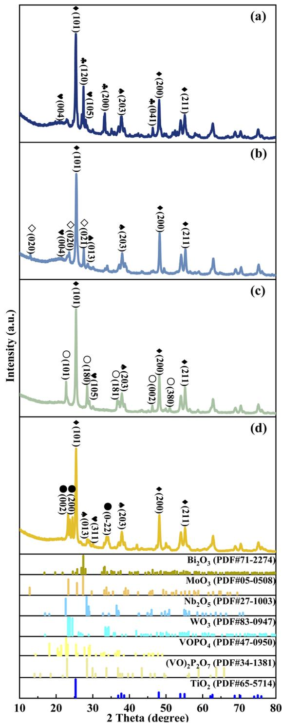
Fig. 3 XRD patterns of metal cation-doped VPO catalysts: (a) VTi-Bi, (b) VTi-Mo, (c) VTi-Nb, and (d) VTi-W. ♣ Bi<sub>2</sub>O<sub>3</sub>, ◇ MoO<sub>3</sub>, ○ Nb<sub>2</sub>O<sub>5</sub>, ● WO<sub>3</sub>, ◆ TiO<sub>2</sub>, ♥ VOPO<sub>4</sub>, ♠ (VO)<sub>2</sub>P<sub>2</sub>O<sub>7</sub>.
