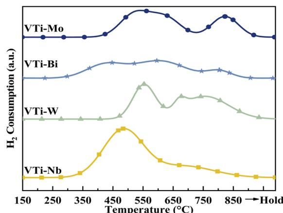
Fig. 7 H<sub>2</sub>-TPR profiles of metal cation-doped VPO catalysts.
