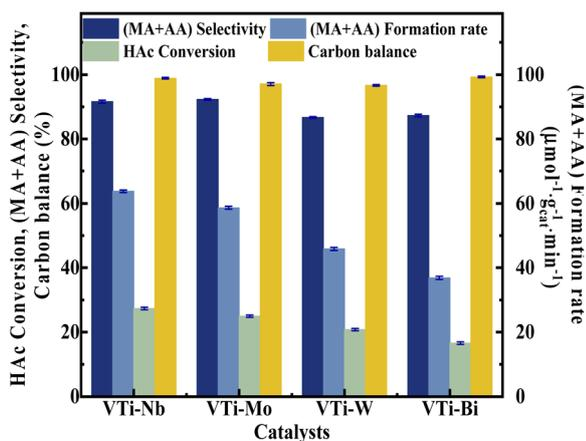
Fig. 8 Catalyst performance of metal cation-doped VPO catalysts. The reaction temperature and carrier flow rate was  $360 \text{ }^\circ\text{C}$  and  $50 \text{ mL min}^{-1}$  ( $3.0 \text{ vol}\% \text{ O}_2$  in  $\text{N}_2$ ), respectively. The liquid feed was a HAC-FA mixture (2.5/1,  $n/n$ ), with a LHSV of  $1.33 \text{ mL h}^{-1} \text{ g}_{\text{cat}}^{-1}$ .
