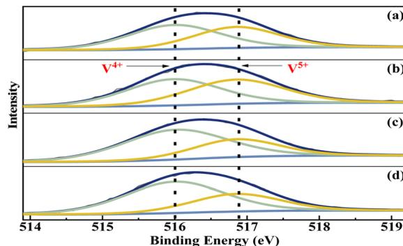
Fig. 5 V 2p<sub>3/2</sub> curve fitting analysis of metal cation-doped VPO catalysts: (a) VTi-Bi, (b) VTi-Mo, (c) VTi-Nb, and (d) VTi-W.
