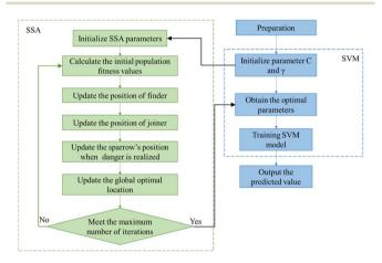
Fig. 1 The working flow chart of the SSA-SVM model.
