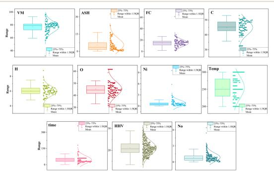
Fig. 2 The statistical distribution of each variable involving the inherent properties of the raw biomass, the torrefaction conditions, and the HHV and No of torrefied biomass.
