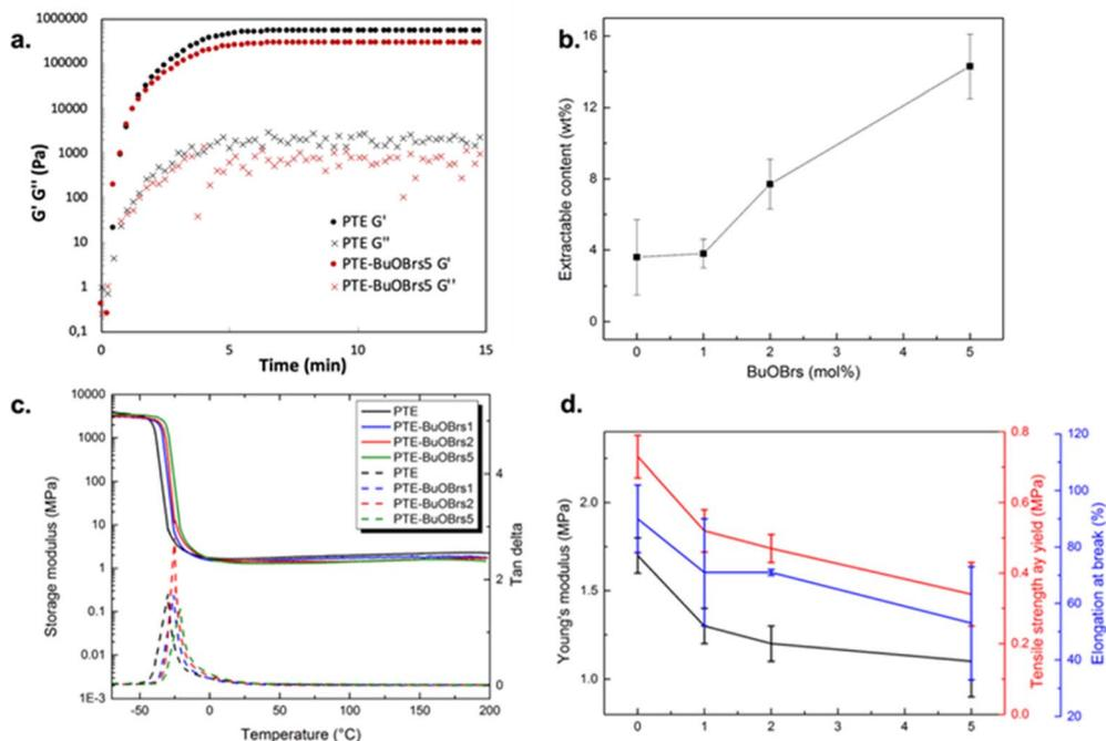
**Fig. 1** (a) Rheological properties of PTE-BuOBrs5 and PTE precursor mixtures as a function of time during photopolymerization; (b) soluble fractions of PTE-BuOBrs samples after thermal treatment at 140 °C for 1.5 h as a function of alkylation agent content; (c) DMA curves of PTE-BuOBrs series samples and PTE control sample; (d) Young's modulus, tensile strength at yield and elongation at break extracted from the stress-strain test as a function of BuOBrs mol% of PTE-BuOBrs samples.
