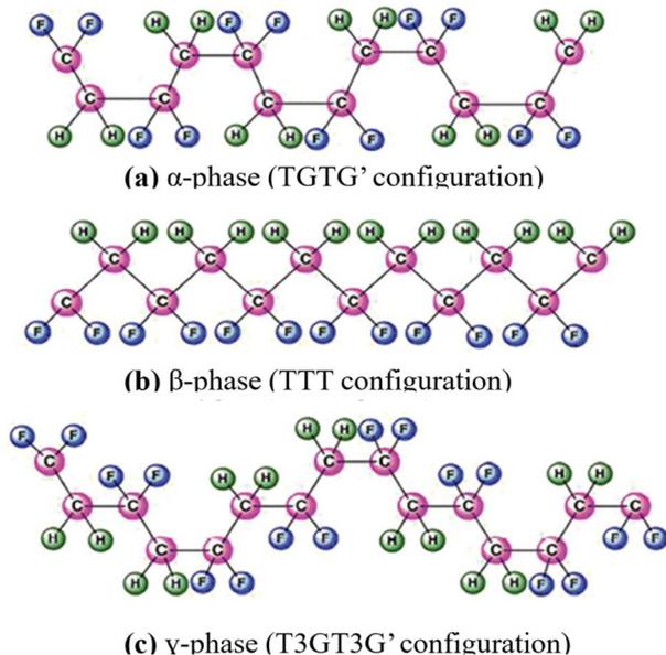
Fig. 3 Chemical structure of the three main phases of PVDF.<sup>20</sup>
