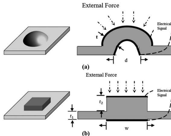
Fig. 20 Scheme and operating principle of the dome/bump-shaped flexible PVDF-TrFE tactile sensors: (a) dome shaped, (b) bump shaped.<sup>50</sup>
