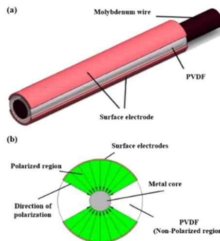
Fig. 22 (a) The structure of the SMPF. (b) The cross-section of the SMPF and polarization distribution.<sup>53</sup>
