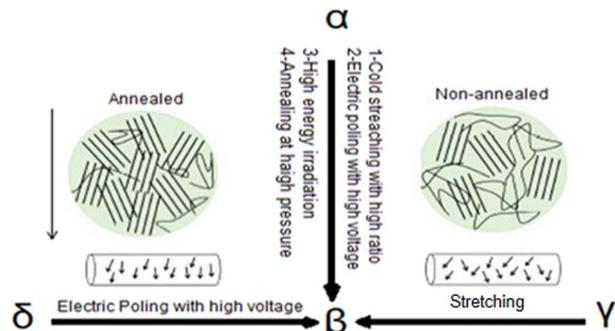
Fig. 6 Mutual transformation routes and fabrication methods of different  $\beta$ -PVDF.<sup>37</sup>
