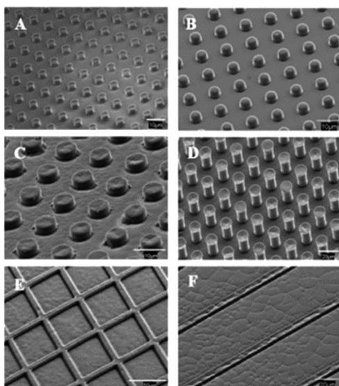
Fig. 17 SEM images of (A and B) singular and (C and D) embossed columns, (E) crisscrossed, and (F) parallel channels.<sup>51</sup>
