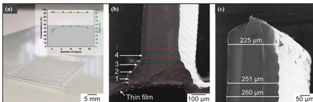
Fig. 12 Images of 3D-printed PVDF–TrFE structures: (a) optical image of a layered PVDF–TrFE on top of a thin film, (b) cross-sectional HIM image of the structure, and (c) the top of the structure.<sup>44</sup>
