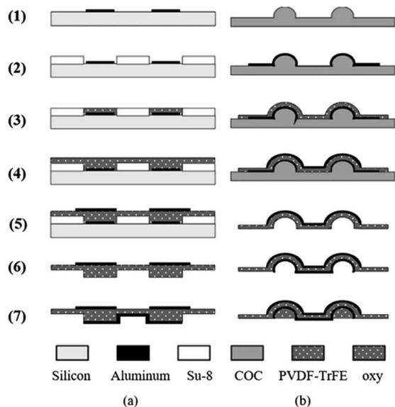
Fig. 18 Summary of soft lithography fabrication steps for bump-shaped films.<sup>50</sup>
