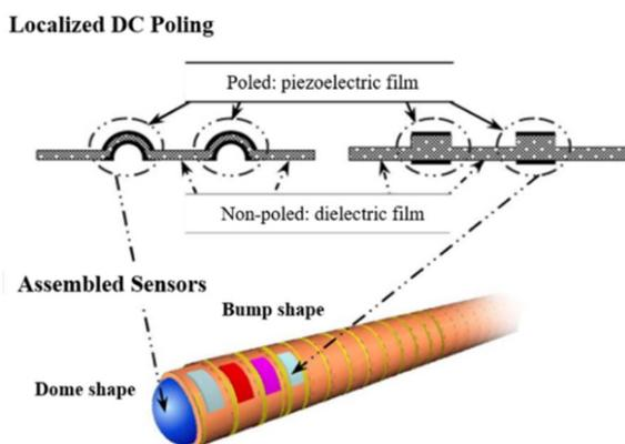
Fig. 19 Schematic of a new mold-transfer method to trim the PVDF-TrFE piezoelectric polymer film and a new dome/bump-shaped tactile sensor module for a smart microcatheter.<sup>50</sup>
