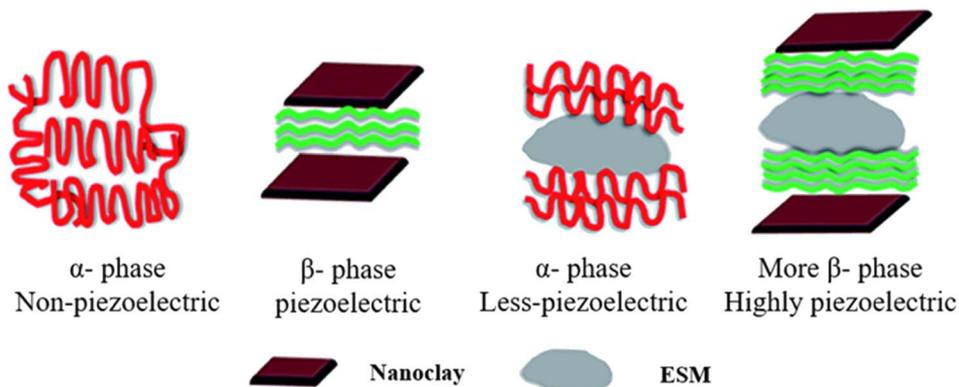
Fig. 23 Schematics of nano-hybrid structural orientations under different conditions with the presence of ESM, nanoclay, and a combination of both.<sup>4</sup>
