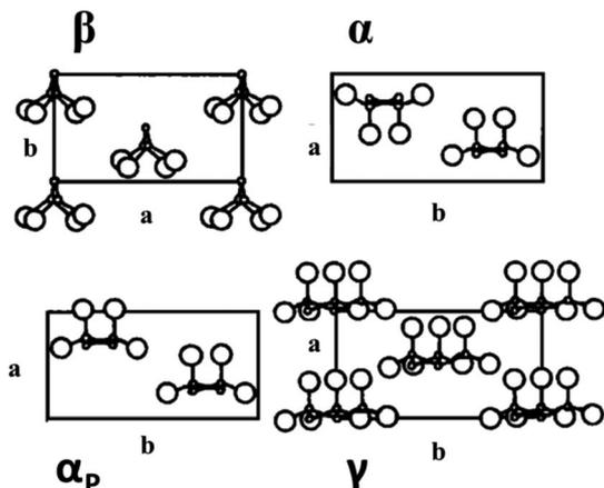
Fig. 2 Crystalline structure of  $\beta$ ,  $\alpha$ ,  $\alpha_p$ , and  $\gamma$  phases of PVDF projected onto the  $a$ - $b$  plane of the unit cell. Large circles are fluorine atoms, small circles means dot carbon atoms, and hydrogen atoms are omitted.<sup>19</sup>
