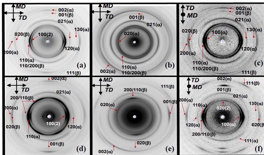
Fig. 11 2D WAXD along the edge, through, and end directions of PVDF:<sup>6</sup> (a) non-oriented along the edge direction, (b) non-oriented along the through direction, (c) non-oriented along the end direction, (d) oriented along with the edge direction, (e) oriented along the end direction.<sup>42</sup>
