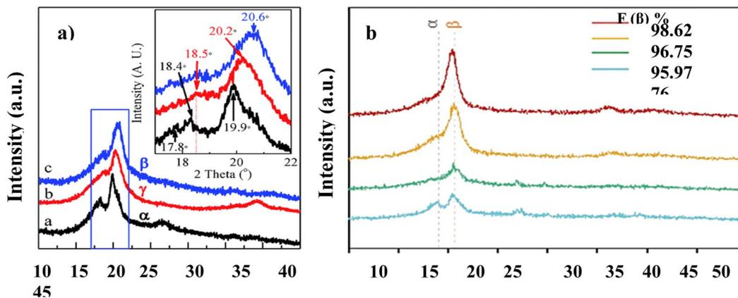
Fig. 10 XRD patterns of the main peak of the crystalline phases of PVDF: (a) oriented,<sup>38</sup> (b) composed.<sup>41</sup>
