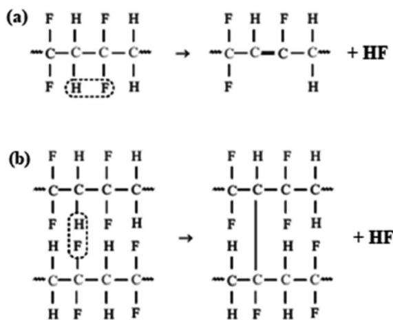
Fig. 4 Schematic diagram of the mechanism of dehydrochlorination in PVDF: (a) formation of double bonds in the chain and (b) cross-linking of the polymer.<sup>16</sup>
