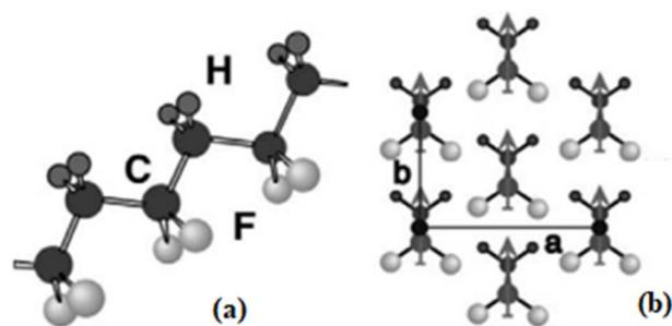
Fig. 1 The structure of PVDF: (a) structure of the all-trans conformations showing the planar carbon backbone with attached fluorine and hydrogen atoms; (b) the crystal structure of the  $\beta$ -phase.<sup>17</sup>
