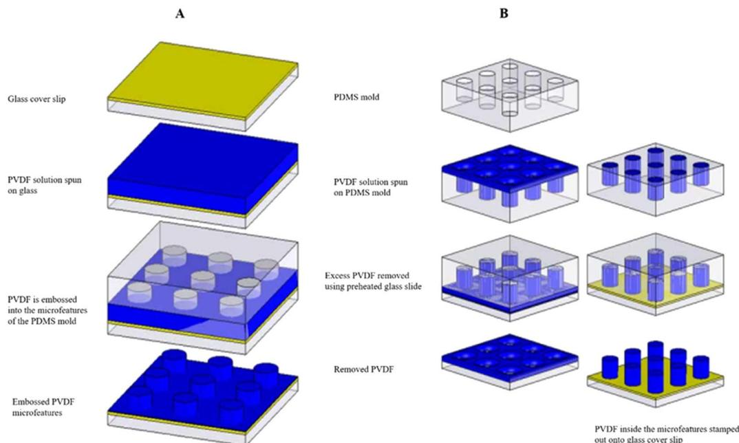
Fig. 16 Illustration of the process of (A) embossed and (B) singular PVDF microstructures.<sup>51</sup>
