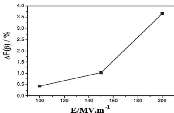
Fig. 7 Evolution of the additional  $\alpha \rightarrow \beta$  phase transformation due to the different corona poling fields.<sup>38</sup>
