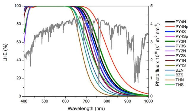
**Fig. 6** LHE curves of all dyes ( $\Gamma = 20 \text{ nmol cm}^{-2}$  is taken for PY-4N, PY-4S, PY-3N, PY-3S,  $\Gamma = 30 \text{ nmol cm}^{-2}$  is considered for the other dyes). AM 1.5G solar spectrum is reported in green.
