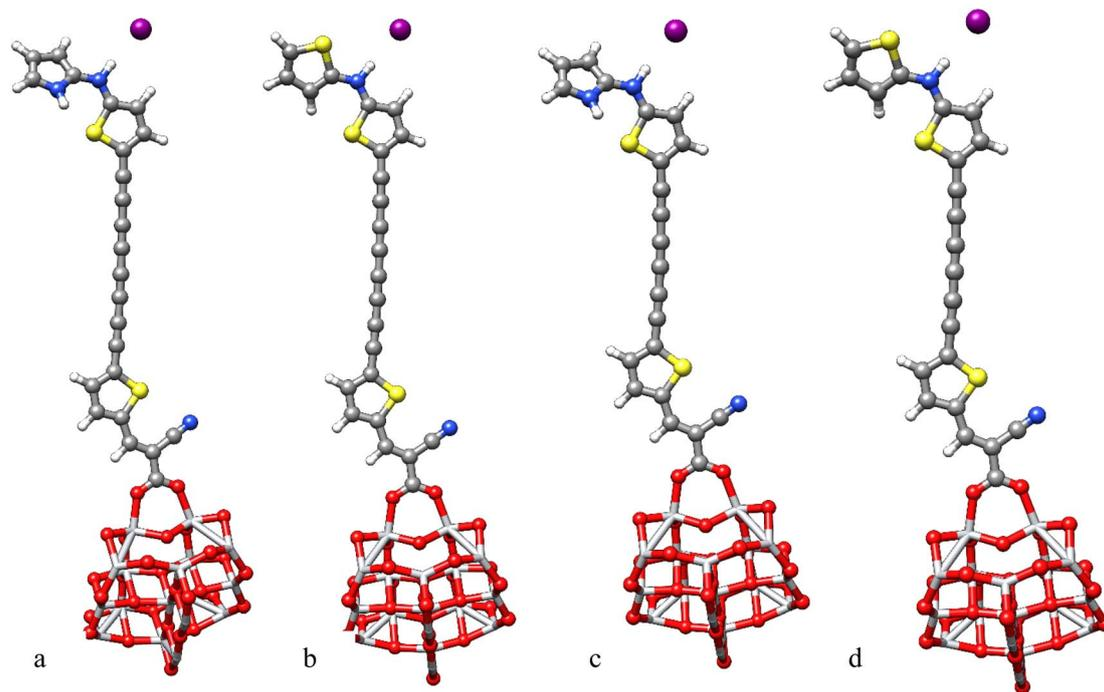
Fig. 9 Optimized geometries of I<sup>-</sup>-PY-4N@(TiO<sub>2</sub>)<sub>14</sub> (a), I<sup>-</sup>-PY-4S@(TiO<sub>2</sub>)<sub>14</sub> (b), I<sup>-</sup>-PY-3N@(TiO<sub>2</sub>)<sub>14</sub> (c), I<sup>-</sup>-PY-3S@(TiO<sub>2</sub>)<sub>14</sub> (d) at B3LYP-D3/6-31G(d)/LANL2DZ/SDDALL level.
