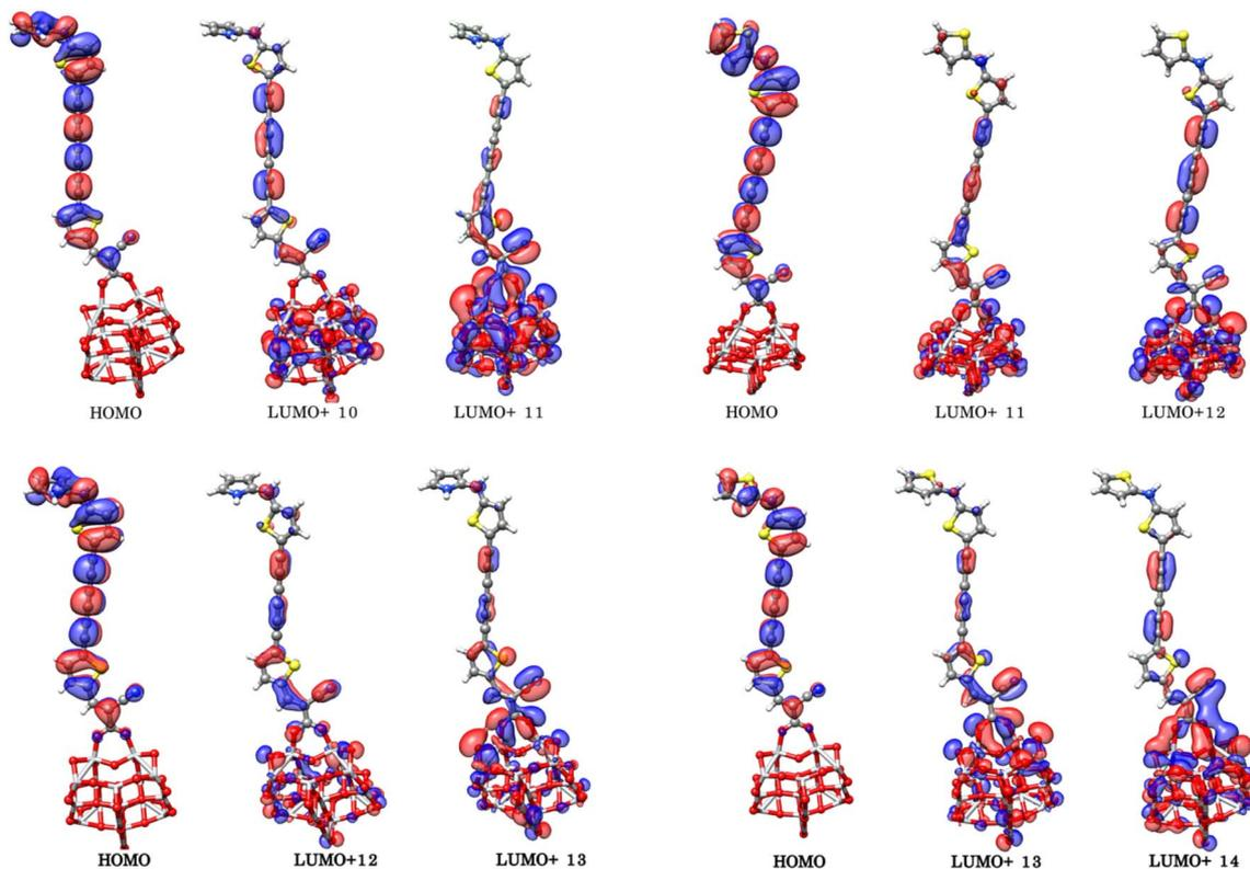
**Fig. 8** Electronic transitions of **PY-4N**@(TiO<sub>2</sub>)<sub>14</sub> (up left), **PY-4S**@(TiO<sub>2</sub>)<sub>14</sub> (up right), **PY-3N**@(TiO<sub>2</sub>)<sub>14</sub> (down left) **PY-3S**@(TiO<sub>2</sub>)<sub>14</sub> (down right) calculated at TD-M062X/6-31G(d)/LANL2DZ level.
