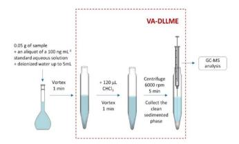
Fig. 1 Schematic diagram of the proposed method
