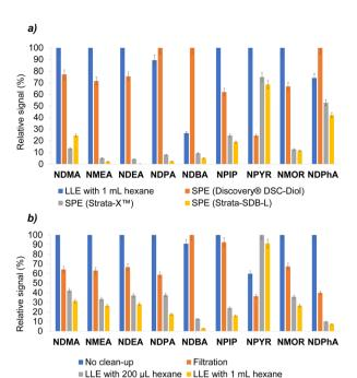
Fig. 3 Sample pretreatment studies carried out with a N-nitrosamine free sample solution spiked to 1 ng mL $^{-1}$  with target analytes: (a) comparison between clean-up through LLE with 1 mL hexane and SPE with different cartridges; (b) comparison between clean-up through LLE with 1 mL and 200  $\mu$ L of hexane, filtration, and no clean-up step with increasing of the extraction solvent volume (*i.e.*, 120  $\mu$ L of chloroform).
