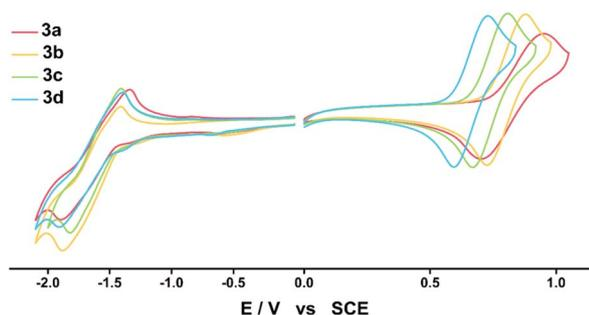
Fig. 2 Cyclic voltammograms of 3a–3d in DCM (left) and in THF (right) recorded at room temperature under argon atmosphere (1 mM/0.1 M TBAP/50 mV s<sup>−1</sup>).
