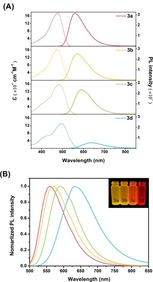
Fig. 1 (A) UV-vis absorption (left) and emission (right) spectra of compounds **3a–3d** in DCM solution at 1  $\mu\text{M}$ . (B) Normalized emission spectra of compounds **3a–3d** (Inset: fluorescence photographs of **3a–3d** in DCM solvent under the irradiation of 365 nm UV light).
