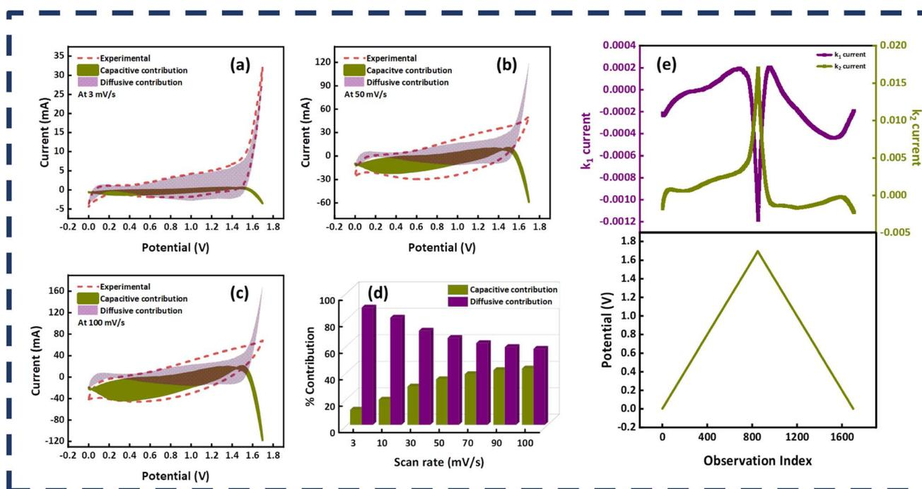
Fig. 9 (a) Capacitive-diffusive contribution of the hybrid device at  $3 \text{ mV s}^{-1}$  extracted through Dunn's model in the potential window of 0–1.6 V. (b) Capacitive-diffusive contribution of the hybrid device at  $50 \text{ mV s}^{-1}$ . (c) Capacitive-diffusive contribution of the hybrid device at  $100 \text{ mV s}^{-1}$ . (d) Capacitive-diffusive percentage contribution at various scan rates. (e)  $k_1$  and  $k_2$  calculated for the hybrid device using Dunn's model.
