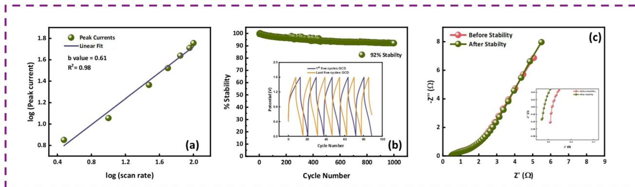
Fig. 8 (a)  $b$ -Values calculated for HKUST-PANI showing the hybrid nature of the device. (b) HKUST-PANI//AC cyclic stability with inset showing the first and last five cycles of the stability test. (c) EIS before and after the stability test of HKUST-PANI//AC.
