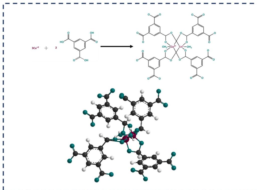
Fig. 1 Structure of the octahedral MOF-199.
