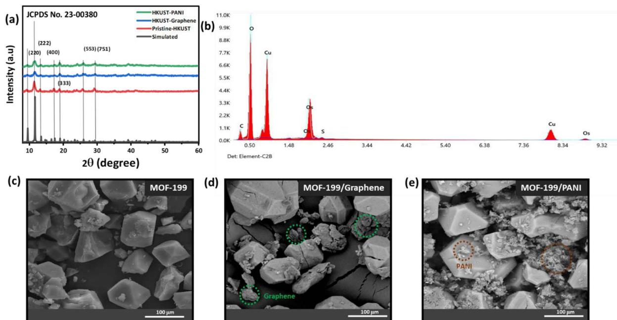
Fig. 2 (a) XRD, (b) EDX and (c–e) SEM micrographs of pristine MOF-199, MOF-199/graphene and MOF-199/PANI.
