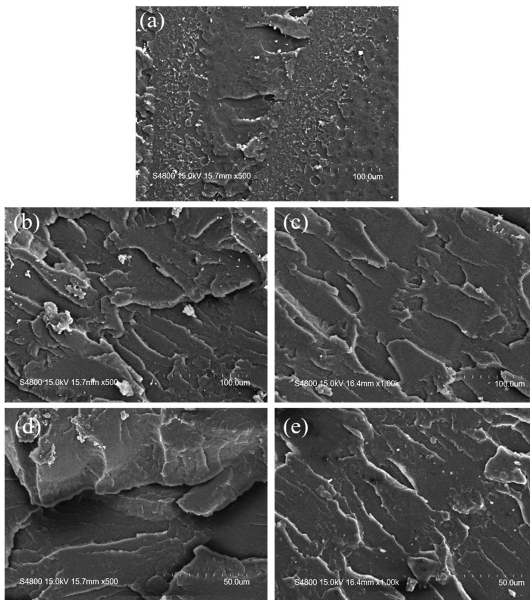
Fig. 8 SEM photographs of the fracture surface of the reactive extrusion PMMA impact specimens: (a) PMMA, (b) blend PMMA/5%CSR, (c) PMMA-5CSR, (d) blend PMMA/15%CSR, (e) PMMA-15CSR.
