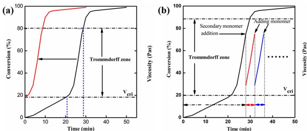
Fig. 1 Schematic diagram for utilizing the Trommsdorff effect.
