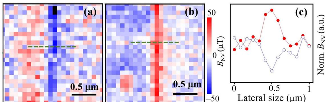
Fig. 5  $B_{\text{NV}}$  map for  $-0.4$  T (a) and  $+0.4$  T (b) field cooled AFM states showing a magnetic field reversible edge DW. (c) Transverse cut of the  $B_{\text{NV}}$  maps in (a) and (b) showing the spatial profile of the edge DW.
