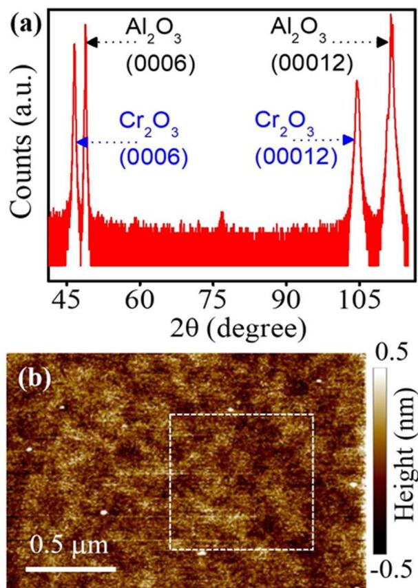
Fig. 1 (a) XRD pattern showing the  $\text{Cr}_2\text{O}_3$  (0006) and  $\text{Al}_2\text{O}_3$  (00012) peaks. (b) Atomic force microscopy topography image of the  $\text{Cr}_2\text{O}_3$  (0001) film surface.
