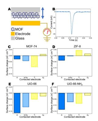
Fig. 2 (A) Schematic of test setup used to determine the charge density of MOFs and (B) current peak generated during contact-separation of Al and UiO-66-NH<sub>2</sub>. Charge density of (C) MOF-74, (D) ZIF-8, (E) UiO-66 and (F) UiO-66-NH<sub>2</sub> after contact-separation against Al, Ni-Mo, Ti and Ag electrodes.
