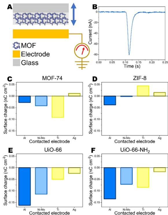
Fig. 2 (A) Schematic of test setup used to determine the charge density of MOFs and (B) current peak generated during contact-separation of Al and UiO-66-NH<sub>2</sub>. Charge density of (C) MOF-74, (D) ZIF-8, (E) UiO-66 and (F) UiO-66-NH<sub>2</sub> after contact-separation against Al, Ni-Mo, Ti and Ag electrodes.
