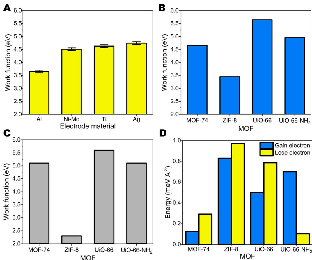
Fig. 1 (A) The measured work function of Al, Ni–Mo, Ti and Ag electrodes; (B) the calculated work function of MOF-74, ZIF-8, UiO-66 and UiO-66-NH<sub>2</sub>. (C) The work function of MOF-74, ZIF-8, UiO-66 and UiO-66-NH<sub>2</sub> obtained by UPS measurements. (D) Energy required to add or remove electron to a unit cell of a MOF structure.
