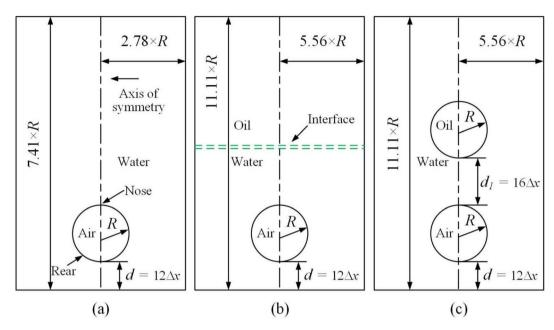
Fig. 1 Schematic of the problem. (a) For Section 3.1 to 3.3, (b) for Section 3.4 and (c) for Section 3.5.
