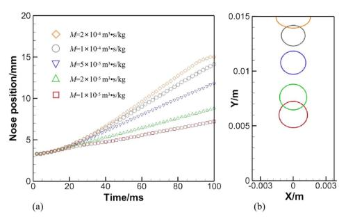
Fig. 10 (a) Effect of the phase field mobility on an air bubble rising in water. (b) Depicts bubble shapes under various phase field mobilities at 100 ms.
