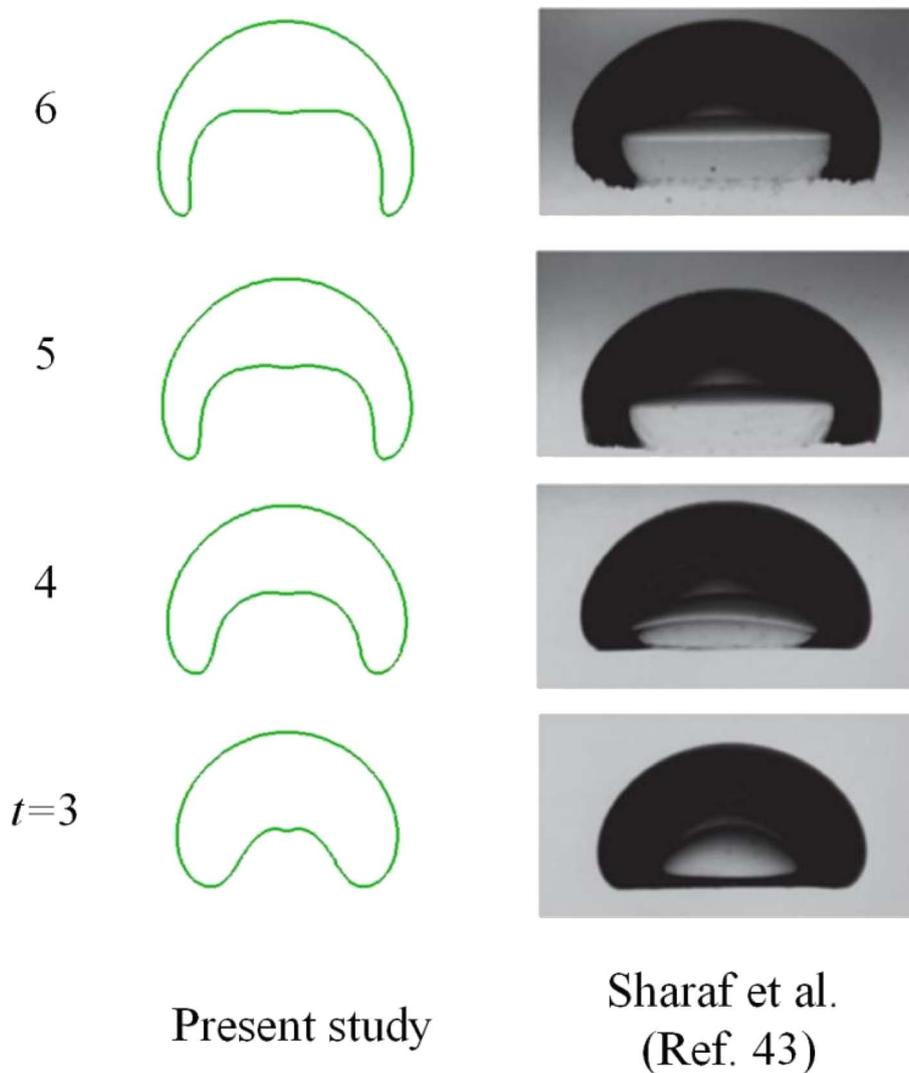
Fig. 8 Comparison of bubble shape with experimental results by Sharaf et al.<sup>43</sup>
