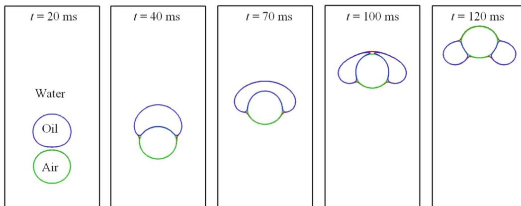
Fig. 16 Bubble–droplet interaction when the air–water and air–oil interfacial tensions are the same.
