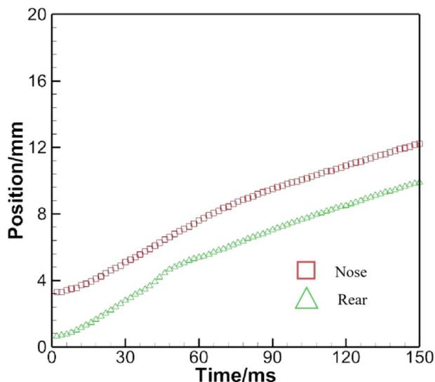
Fig. 13 History of the positions of the nose and rear as a bubble crosses the oil–water interface.
