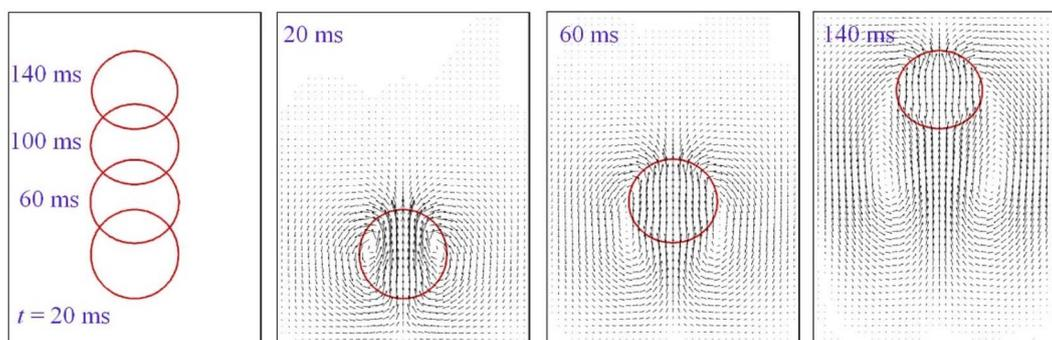
Fig. 6 Bubble shape and velocity field at different instants on the grid of  $\Delta x = 5 \times 10^{-5}$  m.
