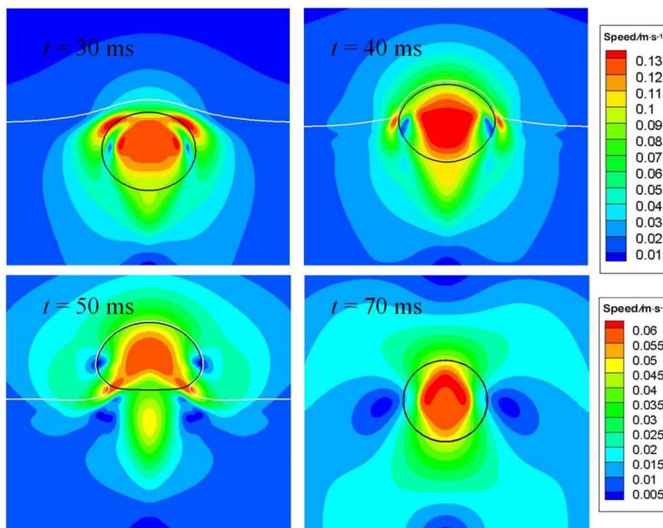
Fig. 12 Flow fields around the air bubble as it is crossing the oil–water interface. The lower scale bar is only for  $t = 70$  ms.
