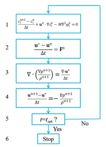
Fig. 3 Flow chart of the algorithm.
