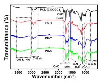
Fig. 1 ATR-FTIR data of PCL-(COOGC)<sub>3</sub>, PU-1, PU-2 and PU-3.
