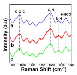
Fig. 2 Raman spectra of the PU film samples (a) PU-1, (b) PU-2 and (c) PU-3.
