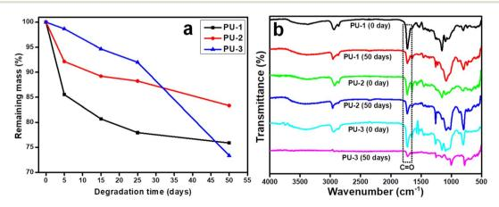
Fig. 11 Degradation studies of the PU films (a) PU-1, PU-2 and PU-3 in PBS (pH = 7.2) medium and (b) the ATR-FTIR spectra of PU-1, PU-2 and PU-3 before and after treated in PBS medium.
