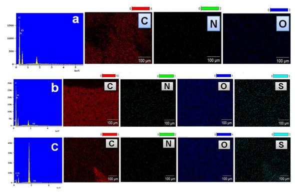
Fig. 13 EDX spectra with elemental mapping for (a) PU-1, (b) PU-2 and (c) PU-3.
