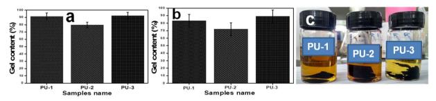
Fig. 8 Cross-link density measurement via the gel content (%) representation in bar diagram, (a) toluene, (b) THF and (c) samples incubated for swelling studies on PU films in THF.
