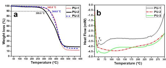
Fig. 7 (a) TGA profiles and (b) DSC curves of PU-1, PU-2 and PU-3.
