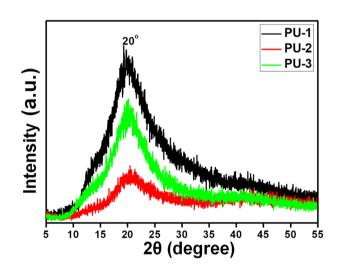
Fig. 6 XRD patterns of PU-1, PU-2 and PU-3
