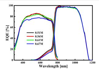
Fig. 7 EQE of the tandem solar cell from various solution concentrations.
