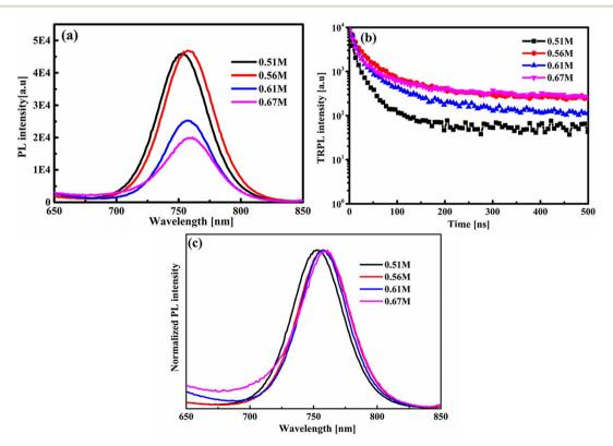
Fig. 5 Perovskite film with different solution concentrations on the silicon heterojunction substrate. Data was collected after perovskite annealing by the same preparation process with a standard tandem cell fabrication sequence. (a) PL spectra (b) TRPL decays data (c) normalized PL spectra.
