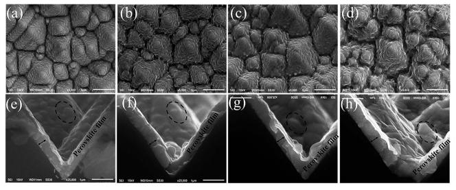
Fig. 6 Surface (a-d) and cross-section (e-h) SEM images of the complete PVSK/SHJ tandem solar cells with solution concentrations of 0.51 M, 0.56 M, 0.61 M, and 0.67 M, respectively.
