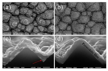
Fig. 2 Surface images (a, b) and cross-section images (c, d) of tandem cells captured by SEM. Where the (a) and (c) without CsBr incorporating, while (b) and (d) contains CsBr (the evaporate rate maintain at  $0.10 \text{ Å s}^{-1}$ ).
