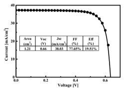
Fig. 10 J-V data of the bottom cell.
