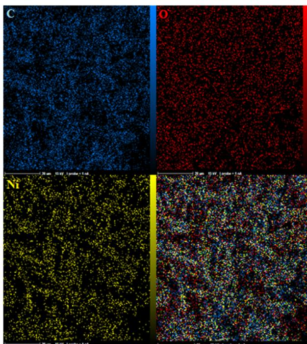
Fig. 4 EDS-mapping of  $\beta$ -CDs/Ni-based MOF composite.
