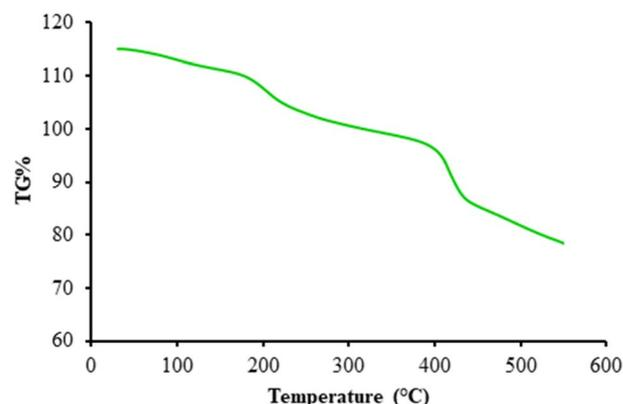
Fig. 5 TGA analysis of  $\beta$ -CDs/Ni-based MOF composite.
