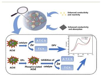
Fig. 2 Schematic diagram of SPCE/GR/AuNPs/AChE/Nafion sensor for OPs detection.
