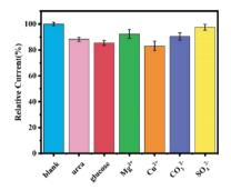
Fig. 10 Current response of SPCE/GR/AuNPs/AChE/Nafion sensors in the presence of different interferents.
