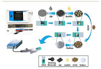
Fig. 1 Preparation process of SPCE/GR/AuNPs/AChE/Nafion.
