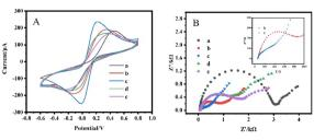
Fig. 4 CV curves (A) and Nyquist diagrams (B) of SPCE/GR/AuNPs/AChE/Nafion electrode assembly process in 5 mM Fe(CN) $_6^{3-/4-}$  (1:1) test solution containing 0.1 M KCl: (a) bare SPCE, (b) SPCE/GR, (c) SPCE/GR/AuNPs, (d) SPCE/GR/AuNPs/AChE, (e) SPCE/GR/AuNPs/AChE/Nafion
