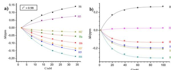
Fig. 6 Concentration effect on the chemical shifts of the NN'-R ligand protons for the  $[\text{Cu}(\text{NN}'\text{-COCH}_3)(\text{PPh}_3)\text{Br}]$  complex at 235 K (a) and for  $[\text{Cu}(\text{NN}'\text{-Cl})(\text{PPh}_3)\text{Br}]$  at 220 K. (b)  $\Delta\delta = \delta_i - \delta_0$ , where  $\delta_i$  correspond to  $\delta$  observed at any concentration and  $\delta_0$  corresponds to the lowest concentration measured.
