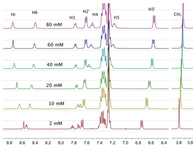
Fig. 5  $^1\text{H-NMR}$  spectra of  $[\text{Cu}(\text{NN}'\text{-OCH}_3)(\text{PPh}_3)\text{Br}]$ ,  $T = 220\text{ K}$ , for several concentrations used to calculate self-association constants. Proton assignment is included. Similar behaviors were observed at different temperatures (see Tables SI3a to g†).
