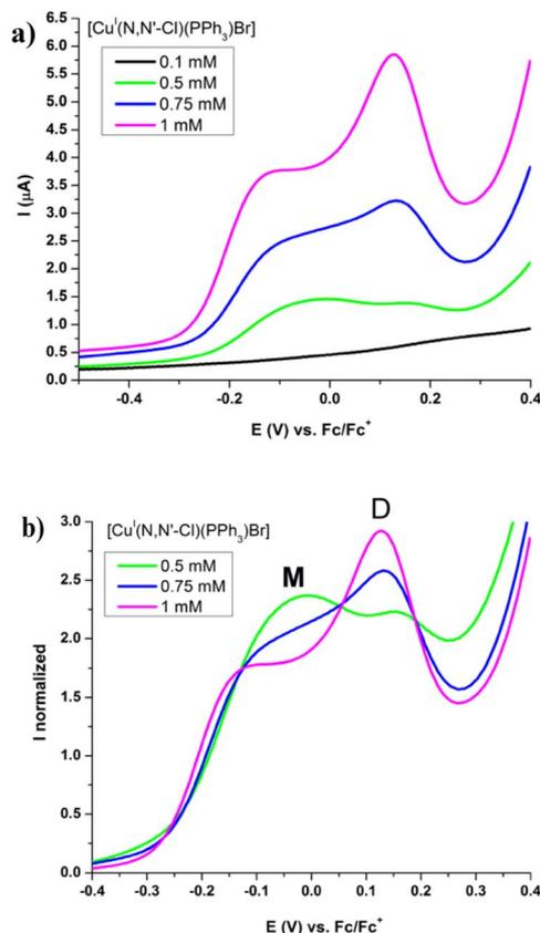
Fig. 9 (top a) SWV of  $[\text{Cu}(\text{NN}'\text{-Cl})(\text{PPh}_3)\text{Br}]$  in  $\text{CH}_2\text{Cl}_2$ , 0.1 M TBAP, 15 Hz, at different initial concentrations. (down b) SWV normalized at absolute area for  $[\text{Cu}(\text{NN}'\text{-Cl})(\text{PPh}_3)\text{Br}]$ , at different initial concentrations. M = monomer; D = dimer.
