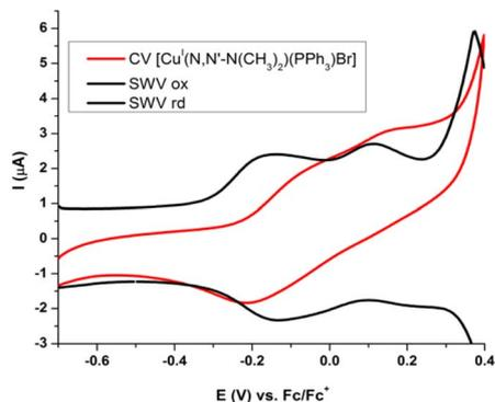
Fig. 8 Cyclic voltammetry and square wave voltammetry of  $[\text{Cu}(\text{NN}'\text{-N}(\text{CH}_3)_2)(\text{PPh}_3)\text{Br}]$  1.0 mM, in  $\text{CH}_2\text{Cl}_2$  and 0.1 M TBAP. SR =  $50 \text{ mV s}^{-1}$  at CV and 15 Hz to SWV.
