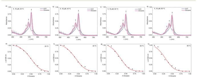
Fig. 2 (a-d) UV-vis spectra of amphiphile 1 in water/dioxane mixtures at different temperatures and  $c_T = 10 \,\mu\text{M}$ . The arrows indicate the changes in the UV-vis spectra upon adding increasing amounts of dioxane. (e-h) Denaturation curves of 1 in water/dioxane mixtures at different temperatures. Red lines depict the fit to the SD model.
