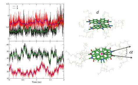
Fig. 4 Time evolution of the selected structural parameters (d and α) computed along the MD trajectory for dimers of N-PBIs 1 and 3. Green and blue lines represent the average values in intervals of 50 points (100 fs). Distance d and angle  $\alpha$  are defined on the right using the dimer of 1.
