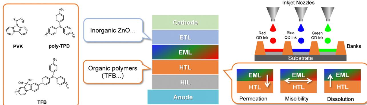
Fig. 2 Challenges in solution-processable HTM-based IJP QD-LEDs.
