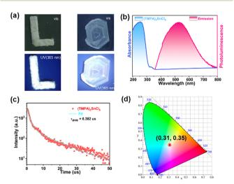
Fig. 3 (a) Crystal and powder of (TMPA)<sub>2</sub>SnCl<sub>6</sub> emit light at 365 nm. (b) Absorption and emission spectra of (TMPA)<sub>2</sub>SnCl<sub>6</sub>. (c) Luminous lifetime of (TMPA)<sub>2</sub>SnCl<sub>6</sub>. (d) CIE chromaticity coordinates of (TMPA)<sub>2</sub>SnCl<sub>6</sub>.
