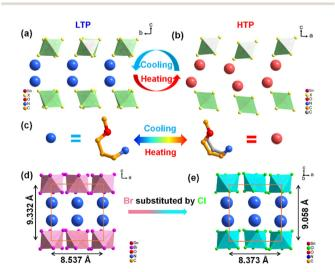
Fig. 2 (a) Molecular structure of  $(TMPA)_2SnX_6$  (X = Cl, Br) at 300 K. (b) Molecular structure of  $(TMPA)_2SnX_6$  (X = Cl, Br) at 380 K. (c) Diagram of ordered and disordered about TMPA. (d) Packing structures of (TMPA)<sub>2</sub>SnCl<sub>6</sub> at 300 K. (e) Packing structures of (TMPA)<sub>2</sub>SnBr<sub>6</sub> at 300 K.
