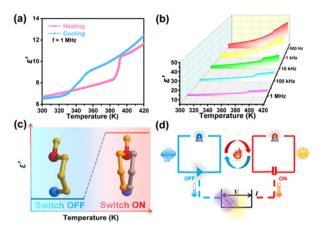
Fig. 5 (a) Dielectric constant of (TMPA)<sub>2</sub>SnCl<sub>6</sub>. (b) Temperature dependence of the real part ( $\epsilon'$ ) of (TMPA)<sub>2</sub>SnCl<sub>6</sub> at different frequencies in the heating run. (c) Scheme of the dielectric switch with a bistable state. (d) Simulated application of the optical/thermal integrated multifunctional switch sensor
