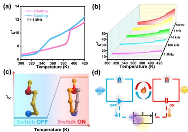
Fig. 5 (a) Dielectric constant of  $(\text{TPMA})_2\text{SnCl}_6$ . (b) Temperature dependence of the real part ( $\epsilon'$ ) of  $(\text{TPMA})_2\text{SnCl}_6$  at different frequencies in the heating run. (c) Scheme of the dielectric switch with a bistable state. (d) Simulated application of the optical/thermal integrated multifunctional switch sensor.
