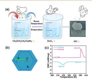
Fig. 1 (a) The synthesis of (TMPA)<sub>2</sub>SnCl<sub>6</sub>. (b) (TMPA)<sub>2</sub>SnCl<sub>6</sub> crystal simulation diagram. (c) DSC curve of (TMPA)<sub>2</sub>SnCl<sub>6</sub> in heating-cooling runs.
