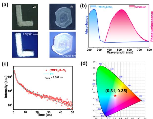
Fig. 3 (a) Crystal and powder of  $(\text{TMPA})_2\text{SnCl}_6$  emit light at 365 nm. (b) Absorption and emission spectra of  $(\text{TMPA})_2\text{SnCl}_6$ . (c) Luminous lifetime of  $(\text{TMPA})_2\text{SnCl}_6$ . (d) CIE chromaticity coordinates of  $(\text{TMPA})_2\text{SnCl}_6$ .
