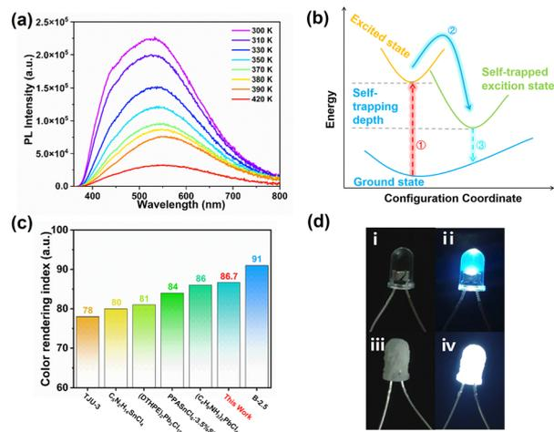
Fig. 4 (a) Temperature-dependent emission spectra of  $(\text{TMPA})_2\text{SnCl}_6$  at the excitation of 337 nm. (b) Diagram of PL mechanism in  $(\text{TMPA})_2\text{SnCl}_6$ . (c) A color rendering index of  $(\text{TMPA})_2\text{SnCl}_6$  compared with tin/lead-based materials. (d) Photographs of LEDs (i) commercial UV-LED and (ii) commercial UV-LED lamps illuminate light (365 nm); the same UV-LED coated with  $(\text{TMPA})_2\text{SnCl}_6$  in the states of turned off (iii) and on (iv).
