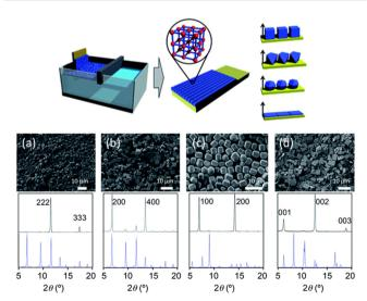
Fig. 14 Scheme of the formation of oriented MOF layers by Langmuir-Blodgettry. SEM images and corresponding out-of-plane XRD patterns of (a) octahedral HKUST-1, (b) cubic HKUST-1, (c)  $[Al_{12}O(OH)_{18}(H_2O)_3-H_1]$  $(Al_2(OH)_4)(BTC)_6]_n$ , and (d)  $[Cu_2(BDC)_2(bpy)]_n$ . Adapted with permission from ref. 103. Copyright 2012, Royal Society of Chemistry.
