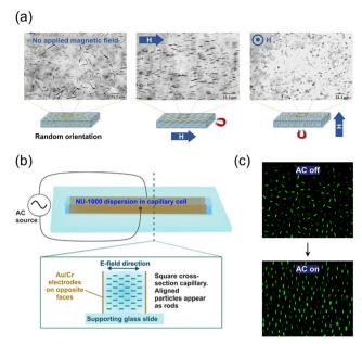
Fig. 12 (a) Alignments of magnetized NH<sub>2</sub>-MIL-53(Al) depending on the direction of the magnetic field. Adapted with permission from ref. 92. Copyright 2017, Wiley-VCH. (b) Setup of a capillary cell and (c) alignments of NU-1000<sub>Si</sub> affected by the electric field. Adapted with permission from ref. 93. Copyright 2019, American Chemical Society.
