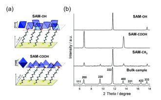
Fig. 5 (a) Schematic illustration of [111] oriented HKUST-1 crystals with -OH SAM and [100] oriented HKUST-1 crystals with the -COOH SAM in the film. (a) XRD patterns of bulk and oriented films of HKUST-1 depending on the SAM functional groups. Adapted with permission from ref. 78. Copyright 2007, American Chemical Society.
