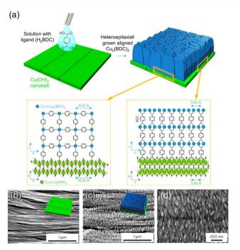
Fig. 3 (a) A schematic illustration inducing the heteroepitaxial growth of  $\text{Cu}_2(\text{BDC})_2$  on 2D substrate of  $\text{Cu}(\text{OH})_2$  by reacting  $\text{H}_2\text{BDC}$  solution with Cu(OH)<sub>2</sub>. SEM images of (b) 2D substrate of Cu(OH)<sub>2</sub> and epitaxially grown Cu<sub>2</sub>(BDC)<sub>2</sub> film on Cu(OH)<sub>2</sub> with (c) low and (d) high magnification. Adapted with permission from ref. 74. Copyright 2017, Springer Nature.
