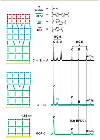
Fig. 6 Schematic diagram depicting the step-by-step hetero-epitaxial growth of SURMOFs with a significant lattice mismatch, accompanied by XRD patterns illustrating the orientation of MOFs at each step. Adapted with permission from ref. 81. Copyright 2014, American Chemical Society.
