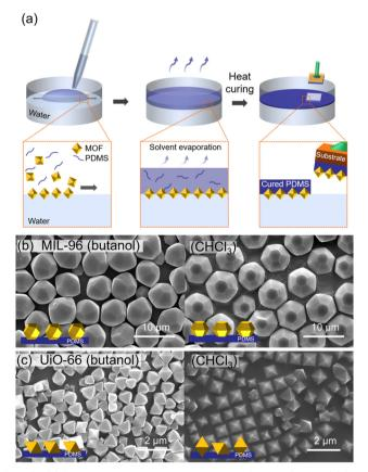
Fig. 16 (a) Scheme of preparation of oriented MOF-PDMS films. (b) SEM images of oriented (b) MIL-96-PDMS films and (c) UiO-66-PDMS films prepared using butanol (left) and CHCl<sub>3</sub> (right) as a casting solvent. Adapted with permission from ref. 101. Copyright 2021, American Chemical Society
