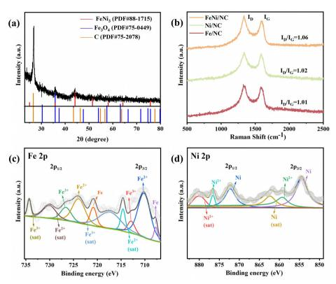
Fig. 2 (a) XRD pattern of FeNi/NC. (b) Raman spectra of FeNi/NC, Fe/NC, and Ni/NC. (c) Fe 2p and (d) Ni 2p XPS spectra of FeNi/NC.
