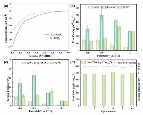
Fig. 3 (a) LSV curves of FeNi/NC measured in Ar and CO<sub>2</sub> saturated 0.1 M KNO<sub>3</sub> electrolytes. (b) The urea yield and (c) urea FE for FeNi/NC, Fe/NC, and Ni/NC on the different applied potentials. (d) The cyclic stability test of FeNi/NC for urea synthesis.
