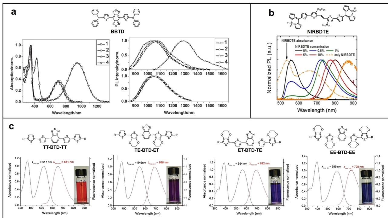
Fig. 2 Chemical structure of BBTD, absorption and emission spectra of (a) BBTD-based compounds; reproduced with permission from ref. 38. Copyright 2009 *Advanced Materials*. (b) NIRBDTE; reproduced with permission from ref. 39. Copyright 2011 *Chemistry of Materials*. (c) TT-BTD-TT, ET-BTD-TE, TE-BTD-ET, and EE-BTD-EE; reproduced with permission from ref. 40. Copyright 2017 *Scientific Reports*.
