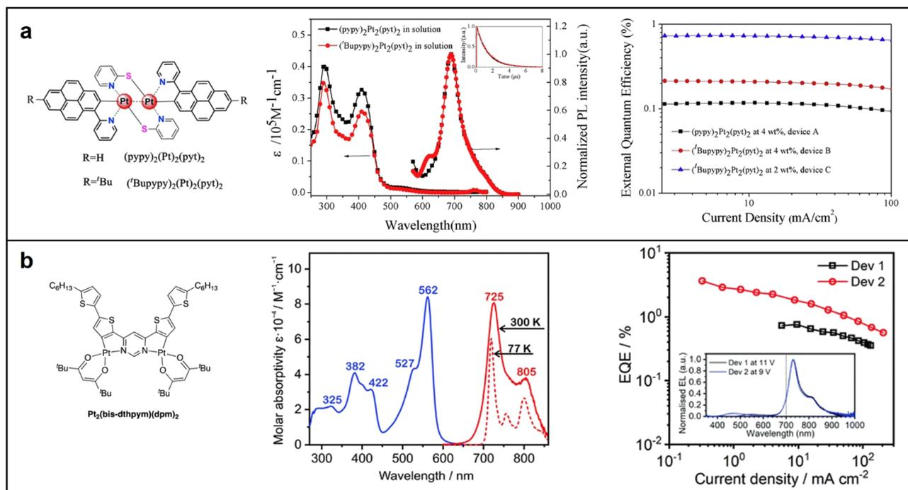
Fig. 7 Chemical structures, absorption and emission spectra, devices EQE of (a) (ppy)<sub>2</sub>Pt<sub>2</sub>(pyt)<sub>2</sub> and (<sup>t</sup>Bupppy)<sub>2</sub>Pt<sub>2</sub>(pyt)<sub>2</sub>; reproduced with permission from ref. 64. Copyright 2017 *Dyes and Pigments*. (b) Pt<sub>2</sub>(bis-dthpym)(dpm)<sub>2</sub>. reproduced with permission from ref. 65. Copyright 2021 *Journal of Materials Chemistry C*.
