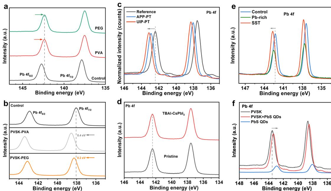
**Fig. 3** XPS spectra of Pb 4f peaks in perovskite films (a) without and (b) with PEG/PVA; (c) before (reference) and after post-treatment by UIPT or APP-PT; (d) CsPbI<sub>3</sub> films before and after TBAI treatment; (e) perovskite films (control), Pb-rich perovskite films (Pb-rich) before and after surface sulfidation treatment (SST-based); (f) pristine PbS QDs, perovskite films without (PVSK) and with PbS QDs (PVSK + PbS QDs).
