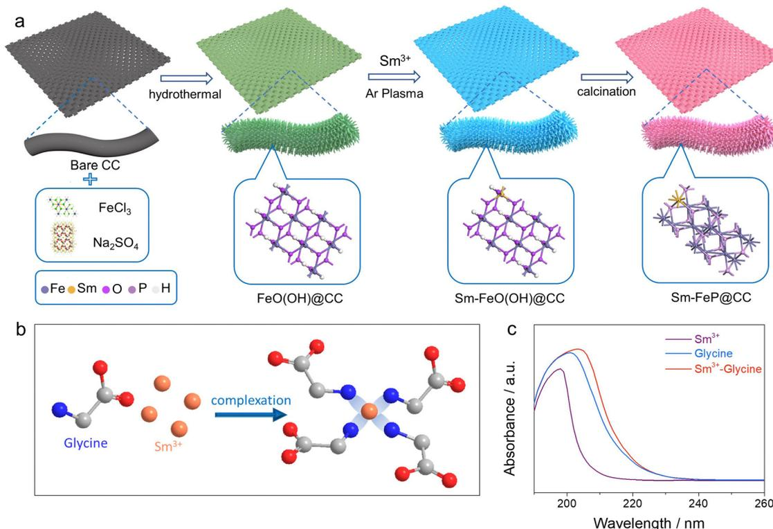
**Fig. 1** (a) A schematic of the fabrication procedure of Sm-FeP@CC; (b) a schematic of the interaction between  $\text{Sm}^{3+}$  and glycine; (c) UV-vis absorption spectra of  $\text{Sm}^{3+}$ , glycine, and  $\text{Sm}^{3+}$ -glycine aqueous solution.
