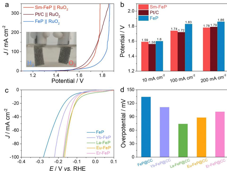
Fig. 6 (a) Polarization curves of Sm-FeP@CC||Pt/C and other counterparts; inset: digital photograph of H<sub>2</sub> and O<sub>2</sub> bubbles during electrolysis; (b) cell voltage comparisons of Sm-FeP@CC||Pt/C and other counterparts at current densities of 10, 100, and 200 mA cm<sup>-2</sup>; (c) comparison of HER polarization curves of different RE-doped FeP@CC in 1 M KOH solution; and (d) overpotentials of different RE-doped FeP@CC at 10 mA cm<sup>-2</sup>.
