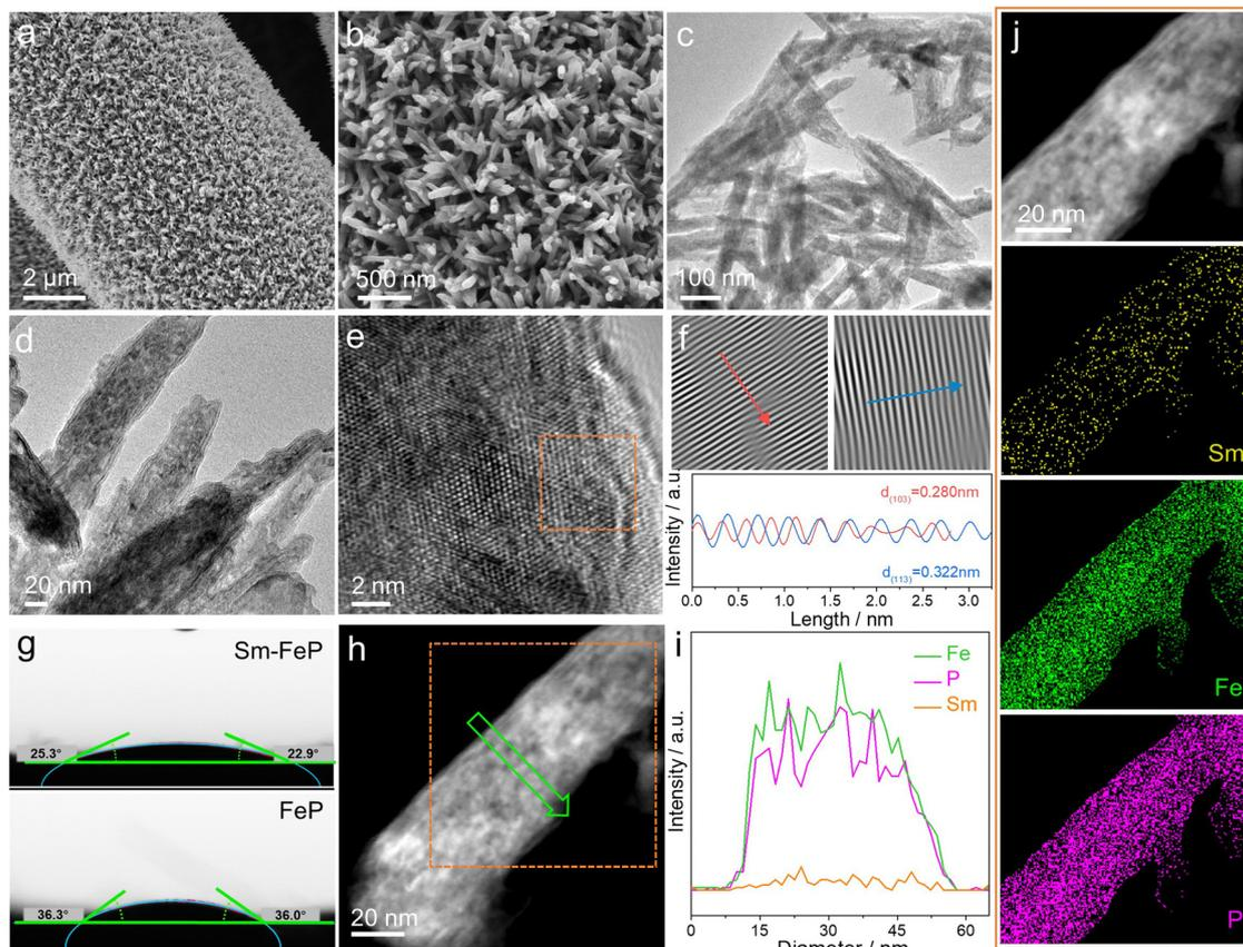
**Fig. 3** Morphology and structure characterization of Sm-FeP@CC: (a), (b) SEM images; (c), (d) TEM images; (e) HRTEM image and (f) HRTEM images after noise elimination and corresponding integrated pixel intensities. (g) Contact angle with a water drop; (h) HAADF-STEM image and (i) EDS line scan profiles. (j) Elemental mapping images.
