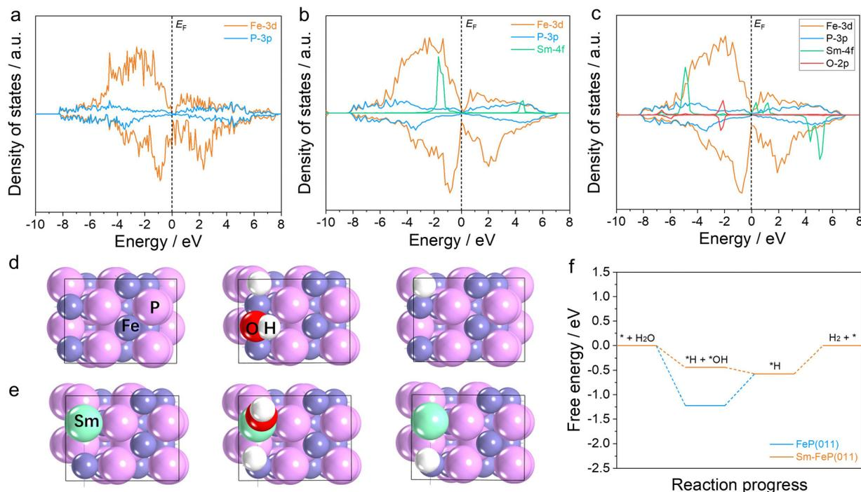
Fig. 5 (a) PDOS of Fe-3d and P-3p in FeP (011); (b) PDOS of Fe-3d, P-3p and Sm-4f in Sm-FeP (011); (c) PDOS of Fe-3d, P-3p, Sm-4f and O-2p in Sm-FeP (011) + (\*H + \*OH); geo-optimized model of (d) FeP and (e) Sm-FeP in the HER; and (f) Gibbs free energy diagram on the Sm-FeP(011) and FeP(011).
