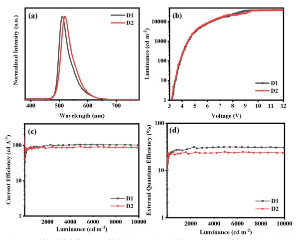
Fig. 3 EL performances of D1 and D2: (a) EL spectra at 6 V, (b) luminance-voltage (L-V) curves, (c) current efficiency-luminance  $(\eta_c-L)$  curves, and (d) external quantum efficiency–luminance (EQE-L) curves.
