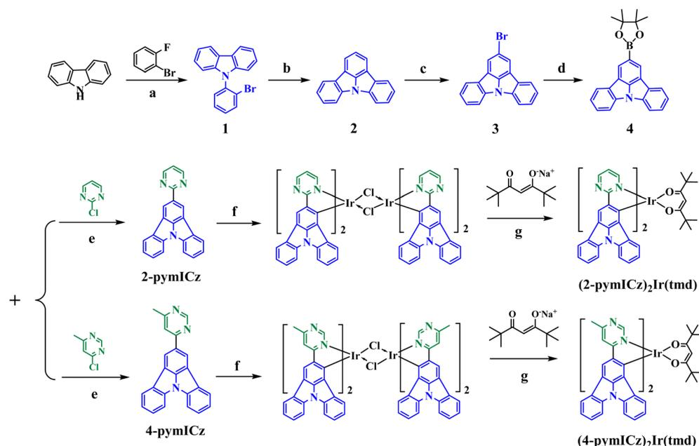
(a): <sup>t</sup>BuOK, DMF, 150 °C, 12 h; (b): Pd(OAc)<sub>2</sub>, K<sub>2</sub>CO<sub>3</sub>, DMAC, 170 °C, 12 h; (c): NBS, DCM, r.t., 12 h; (d): Pd(dppf)Cl<sub>2</sub>, KOAc, Dioxane, 100 °C, 12h;
