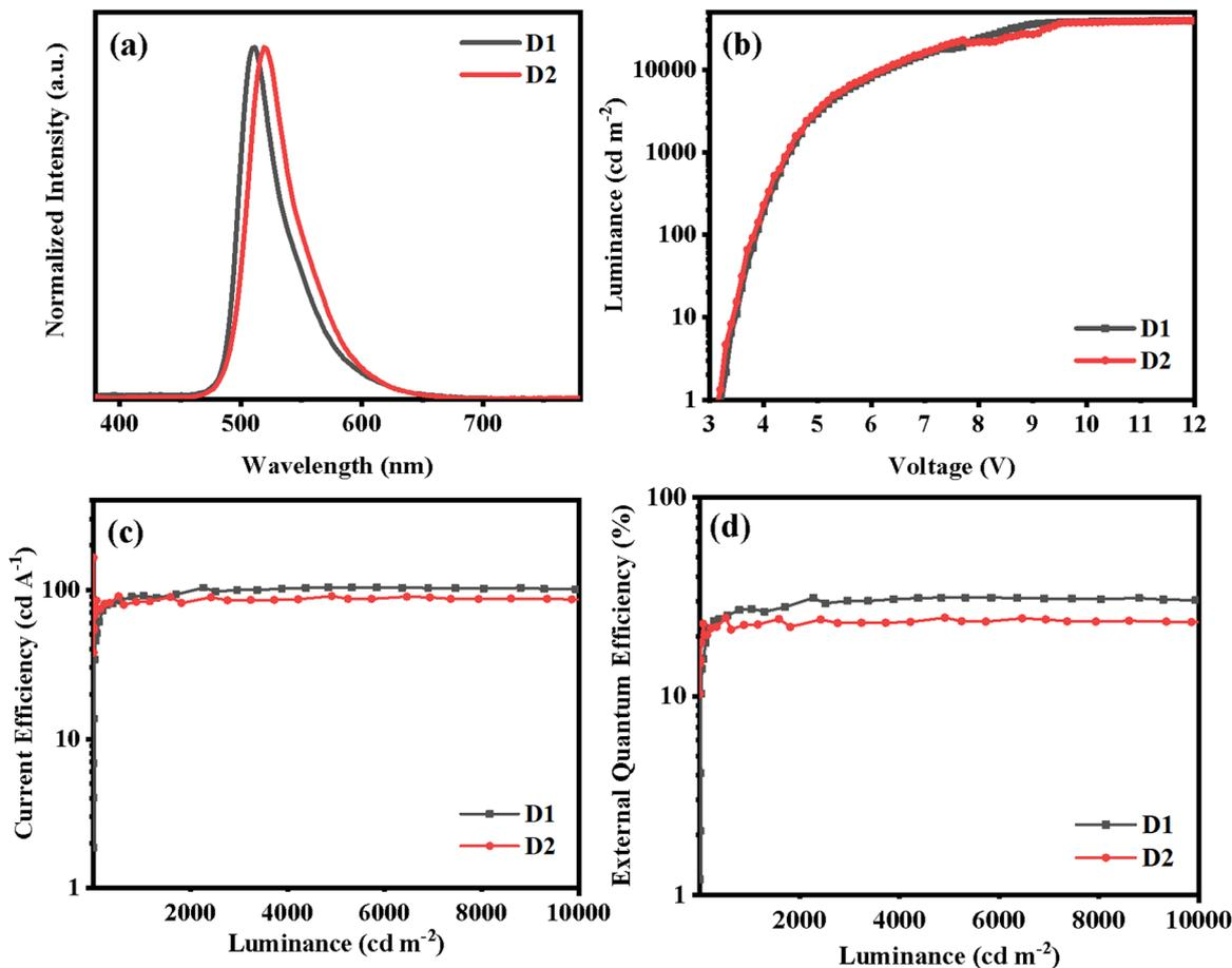
Fig. 3 EL performances of D1 and D2: (a) EL spectra at 6 V, (b) luminance–voltage ( $L$ – $V$ ) curves, (c) current efficiency–luminance ( $\eta_c$ – $L$ ) curves, and (d) external quantum efficiency–luminance (EQE– $L$ ) curves.
