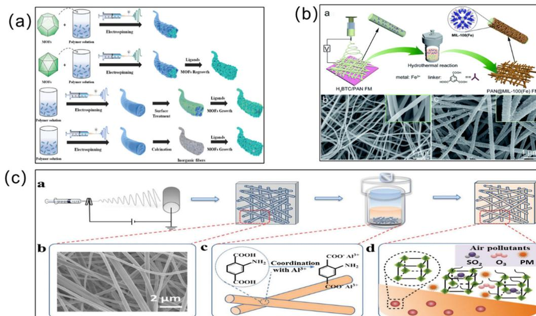
Fig. 9 (a) Schematic diagram of electrospinning for the manufacture of MOF nanofibers (NFs). Reprinted with permission from ref. 99. Copyright 2022 Elsevier. (b) Preparation of the PAN@MIL-100(Fe) fiber membrane via electrospinning. Reprinted with permission from ref. 100. Copyright 2019 Royal Society of Chemistry. (c) Preparation and adsorption process of a MOF-based fiber membrane prepared via electrospinning. Reprinted with permission from ref. 101. Copyright 2019 Royal Society of Chemistry.
