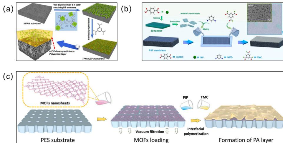
**Fig. 8** (a) Preparation process of a TFN containing PSS-modified ZIF-8 nanoparticles *via* IP. Reprinted with permission from ref. 29. Copyright 2016 American Chemical Society. (b) Schematic illustration for the fabrication of a 2D-MOF-modified TFN membrane *via* the IP reaction. Reprinted with permission from ref. 97. Copyright 2022 Elsevier. (c) Fabrication process for the MOF-interlayered TFN membrane. Reprinted with permission from ref. 98. Copyright 2022 Elsevier.
