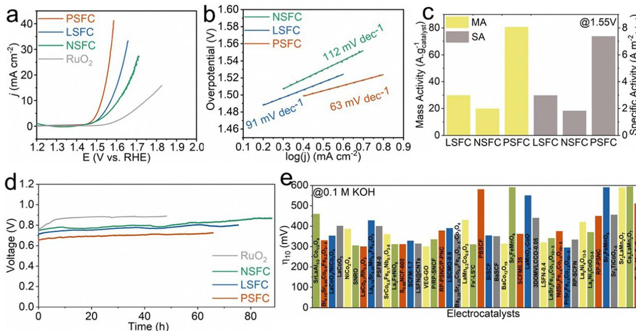
Fig. 2 (a) OER polarization curves of LSFC, NSFC, PSFC, and commercial  $IrO_2$  catalysts in  $O_2$ -saturated 0.1 M KOH. (b) Tafel plots of LSFC, NSFC, and PSFC. (c) Mass activities based on the oxide weight and BET surface area-normalized intrinsic activities of the catalysts at 1.55 V. (d) Chronopotentiometric curves of the catalysts at  $10 \text{ mA cm}^{-2}$ . (e) OER activity comparisons of  $\eta_{10}$  with other reported state-of-the-art catalysts in 0.1 M KOH.
