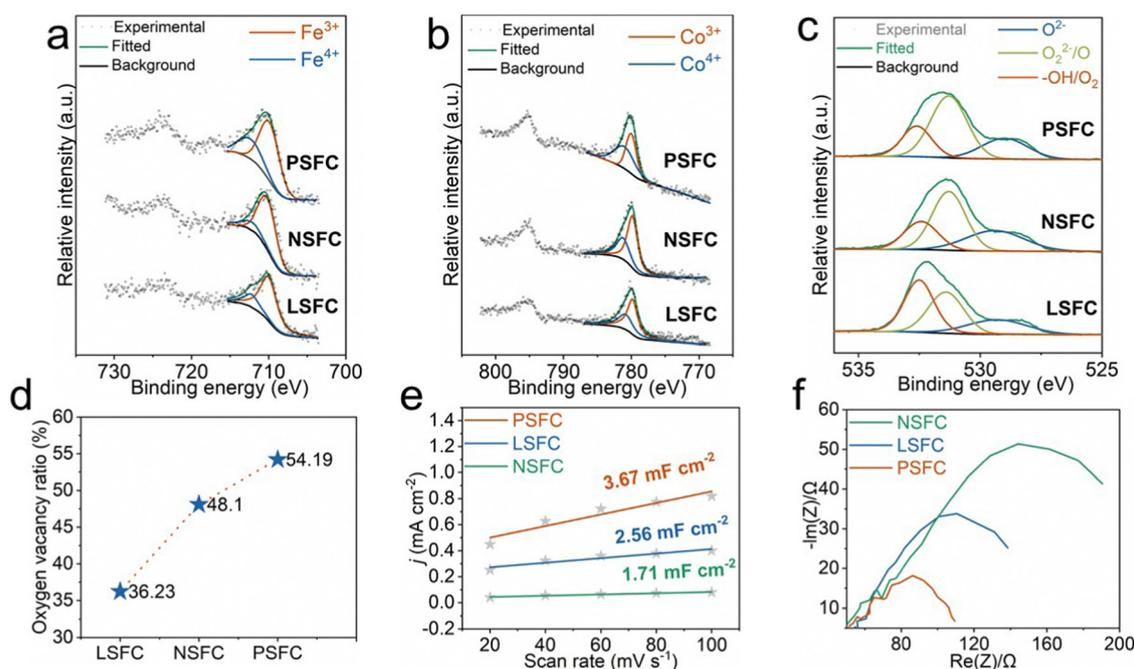
**Fig. 3** (a–c) Fe 2p, Co 2p and O 1s XPS spectra of LSFC, NSFC, and PSFC. (d) The proportion of oxygen vacancies in LSFC, NSFC, and PSFC. (e) Linear fitting of the capacitive currents versus CV scan rates of LSFC, NSFC, and PSFC. (f) EIS spectra of LSFC, NSFC, and PSFC.
