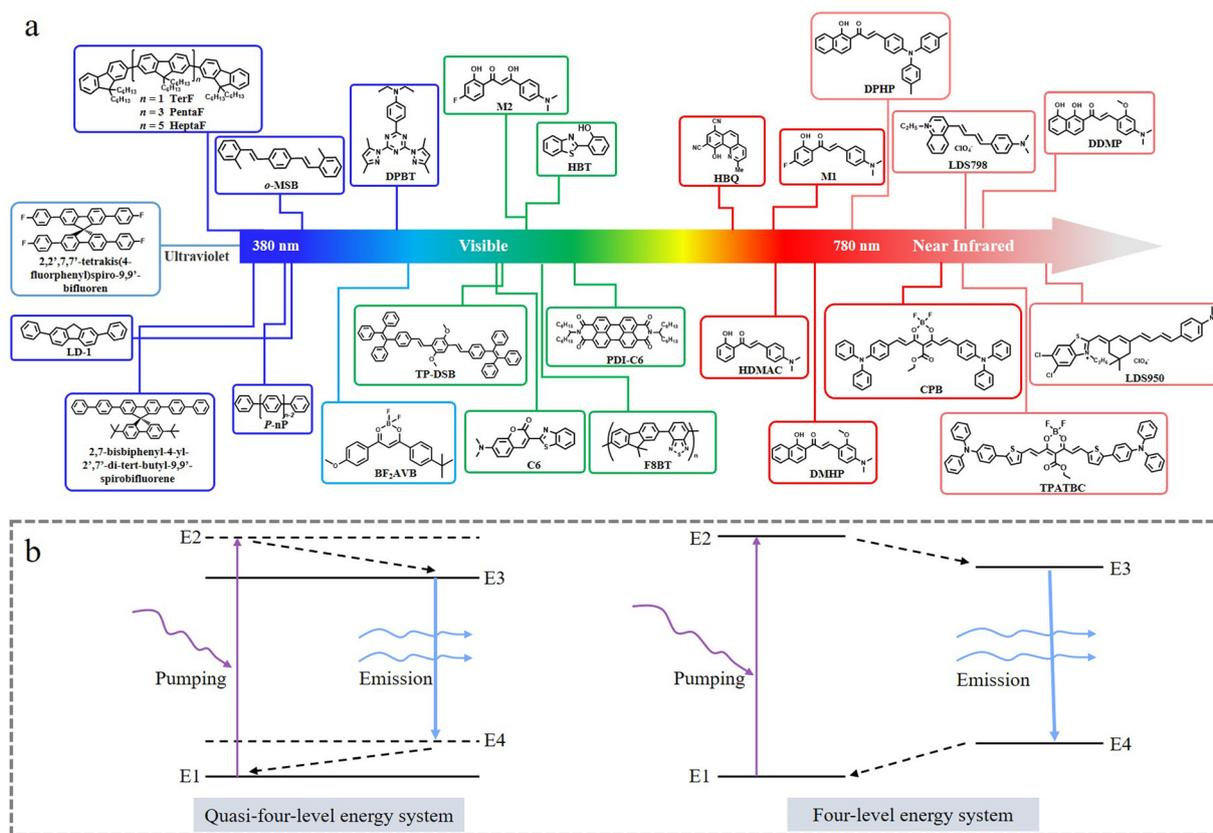
Fig. 2 (a) Molecular structures of typical organic molecule with lasing emissions from ultraviolet to near-infrared. (b) Schematic of the quasi-four-level system (left) and four-level system (right).
