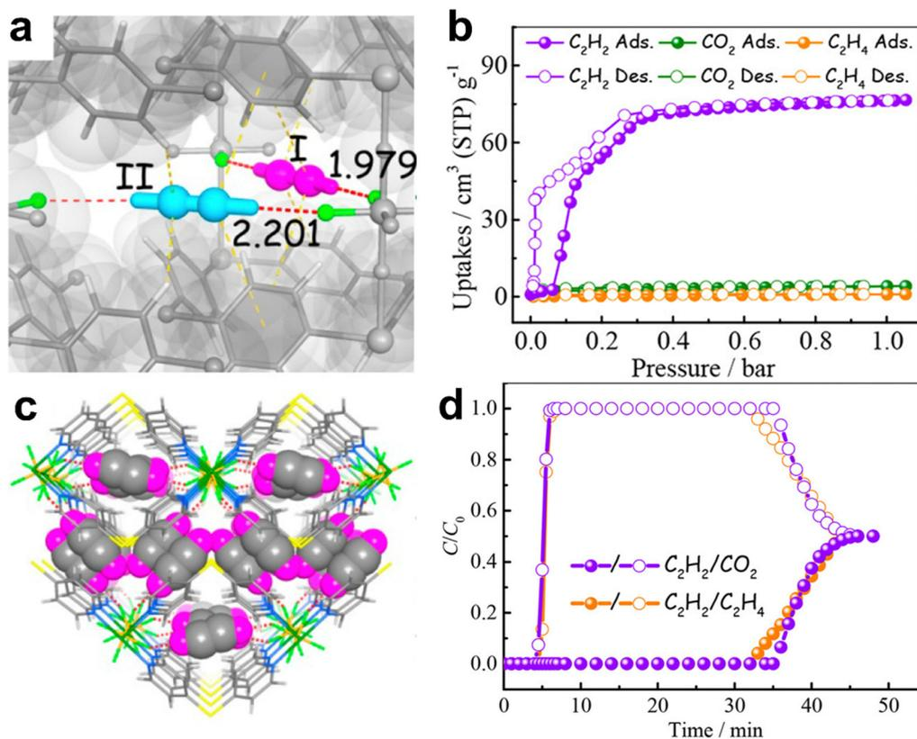
Fig. 9 (a) and (c) Neutron diffraction crystal structure of  $UTSA-300 \supset C_2D_2$  and (b)  $C_2H_2$ ,  $CO_2$ , and  $C_2H_4$  sorption isotherms for UTSA-300a at 273 K. (d) Experimental column breakthrough curves for equimolar  $C_2H_2/CO_2$  (purple) and  $C_2H_2/C_2H_4$  (orange) mixtures (298 K, 1 bar) in a fixed-bed packed with UTSA-300a. Reprinted with permission from ref. 72. Copyright 2017 American Chemical Society.
