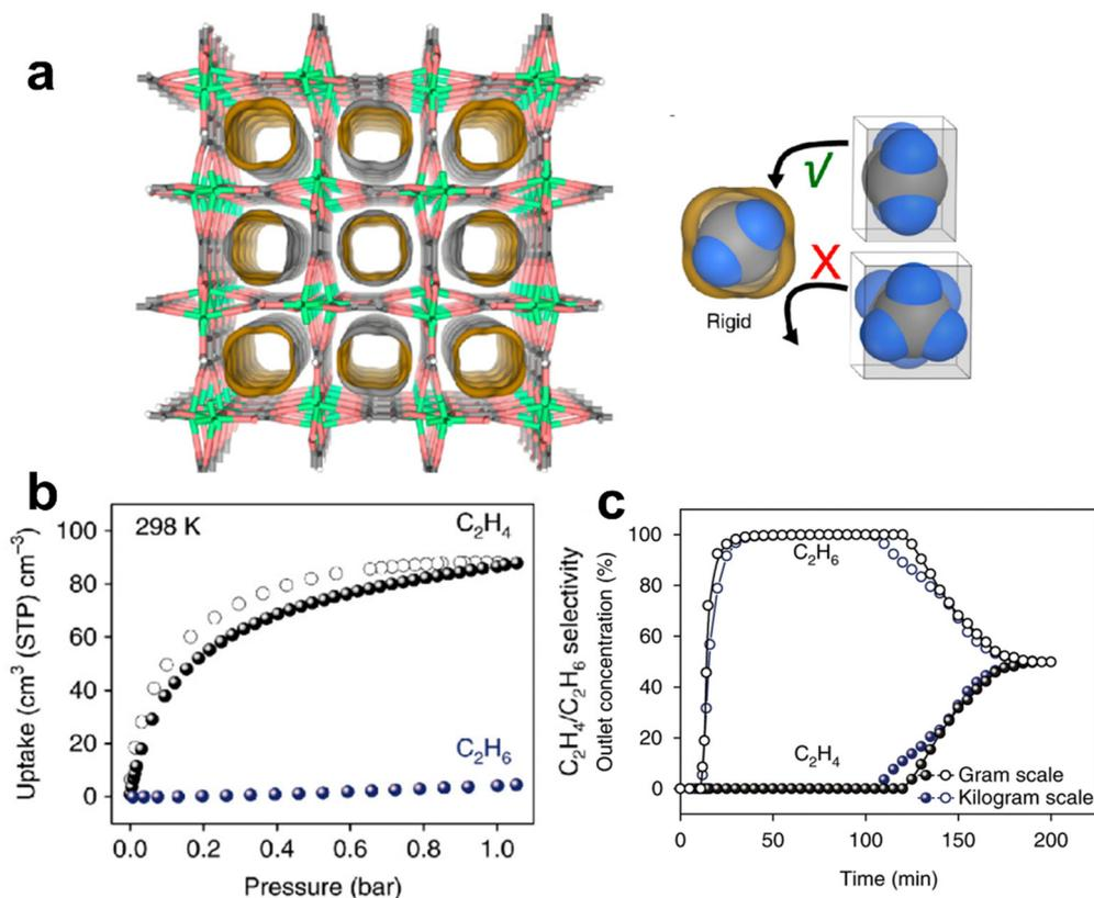
Fig. 2 (a) Structure of UTSA-280. (b) Sorption isotherms of UTSA-280 for  $C_2H_4$  and  $C_2H_6$  at 298 K. (c) Breakthrough curves for UTSA-280 from different scales for an equimolar mixture of  $C_2H_4/C_2H_6$  at 298 K and 1 bar. Reprinted with permission from ref. 35. Copyright 2018 Nature Publishing Group.
