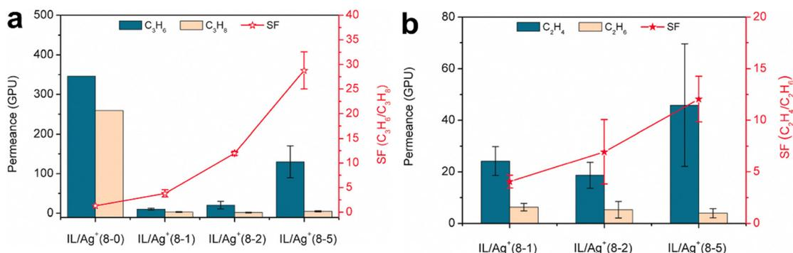
Fig. 24 (a)  $C_3H_6/C_3H_8$  separation performance of  $Zn_2(bim)_4$  membranes modified by diversified composites, IL/Ag<sup>+</sup>(8-0), IL/Ag<sup>+</sup>(8-1), IL/Ag<sup>+</sup>(8-2) and IL/Ag<sup>+</sup>(8-5). (b)  $C_2H_4/C_2H_6$  separation performance of  $Zn_2(bim)_4$  membranes modified by diversified composites, IL/Ag<sup>+</sup>(8-1), IL/Ag<sup>+</sup>(8-2) and IL/Ag<sup>+</sup>(8-5). Reprinted with permission from ref. 217. Copyright 2021 Elsevier.
