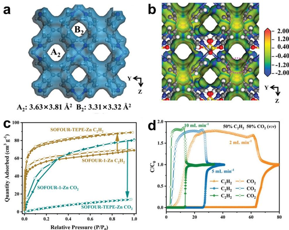
Fig. 10 (a) and (b) The building blocks of SOFOUR-TEPE-Zn and electrostatic surface potential. (c)  $\text{C}_2\text{H}_2$  and  $\text{CO}_2$  adsorption isotherms for SOFOUR-1-Zn and SOFOUR-TEPE-Zn at 298 K. (d) Breakthrough curves of SOFOUR-TEPE-Zn for  $\text{C}_2\text{H}_2/\text{CO}_2$  (50/50, v/v) at different flow rates at 298 K. Reprinted with permission from ref. 97. Copyright 2023 Wiley-VCH.
