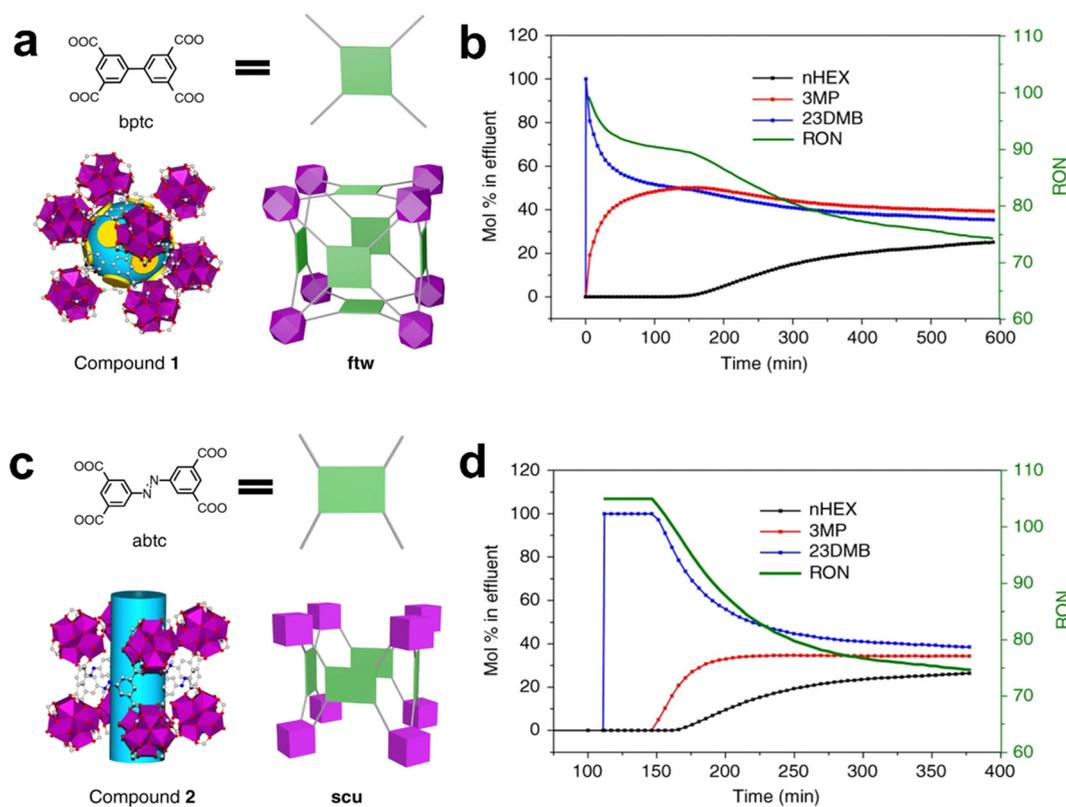
Fig. 21 (a) and (c) Organic ligands, crystal structures, and topologies of Zr-bptc and Zr-abtc. (b) and (d) Breakthrough curves of an equimolar ternary mixture of  $C_6$  alkane isomers at 150 °C for Zr-bptc (top) and Zr-abtc (bottom). The green curve represents the real-time RON of the eluted products. Reprinted with permission from ref. 197. Copyright 2018 Nature Publishing Group.
