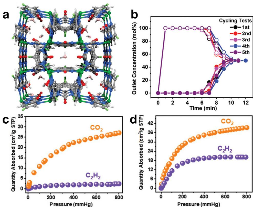
Fig. 11 (a) Schematic structure of Cu-F-pymo MOF with residual water molecules. (b) Breakthrough cycling tests of the equimolar CO<sub>2</sub>/C<sub>2</sub>H<sub>2</sub> mixture. (c) and (d) Separation performance toward CO<sub>2</sub> and C<sub>2</sub>H<sub>2</sub> in Cu-F-pymo under different activation conditions. Reprinted with permission from ref. 143 Copyright 2021 Wiley-VCH.
