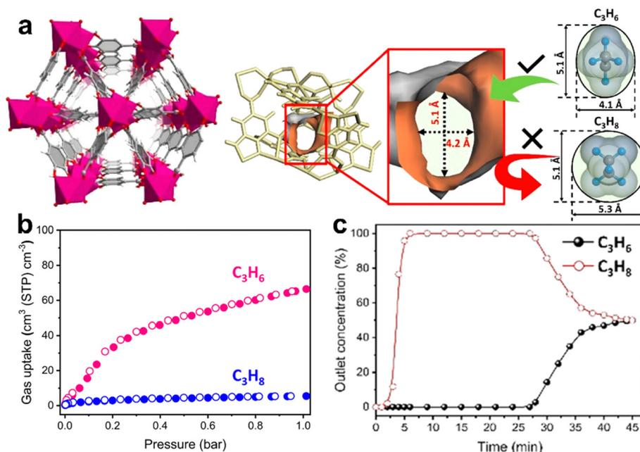
Fig. 15 (a) Structure of the Co-gallate MOF and rationale for C<sub>3</sub>H<sub>6</sub>/C<sub>3</sub>H<sub>8</sub> separation. (b) Gas sorption isotherms of propylene and propane at 298 K for Co-gallate. (c) The breakthrough experiments were carried out in a packed column. Reprinted with permission from ref. 154. Copyright 2020 American Chemical Society.
