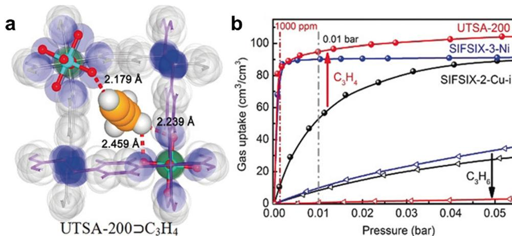
Fig. 19 (a) DFT-D optimized structure and binding sites of  $\text{UTSA-200} \supset \text{C}_3\text{H}_4$ . (b)  $\text{C}_3\text{H}_4$  and  $\text{C}_3\text{H}_6$  adsorption isotherms of UTSA-200 at 298 K. Reprinted with permission from ref. 182. Copyright 2018 Wiley-VCH.
