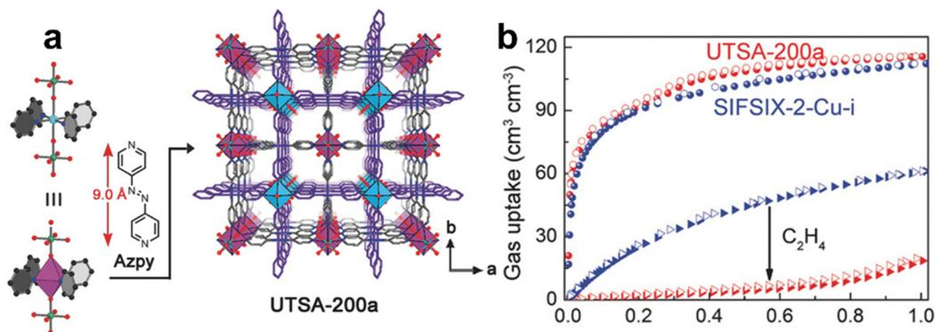
Fig. 7 (a) Crystal structure of UTSA-200. (b) C<sub>2</sub>H<sub>2</sub> and C<sub>2</sub>H<sub>4</sub> adsorption isotherms of UTSA-200a at 298 K. Adapted from ref. 71 with permission from Wiley-VCH, Copyright 2018.
