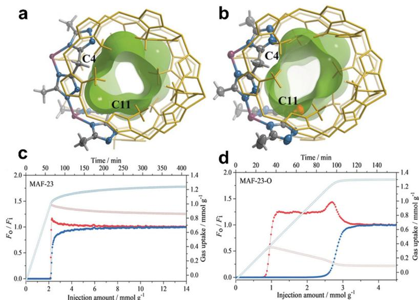
**Fig. 13** Crystal and pore structures of (a) MAF-23 and (b) MAF-23-O. Breakthrough curves (filled symbols) and adsorption kinetic curves (open symbols) for (c) MAF-23 and (d) MAF-23-O using an equimolar  $C_3H_6/C_3H_8$  (blue/red) mixture at 298 K and 1 bar. Reprinted with permission from ref. 149. Copyright 2019 Wiley-VCH.
