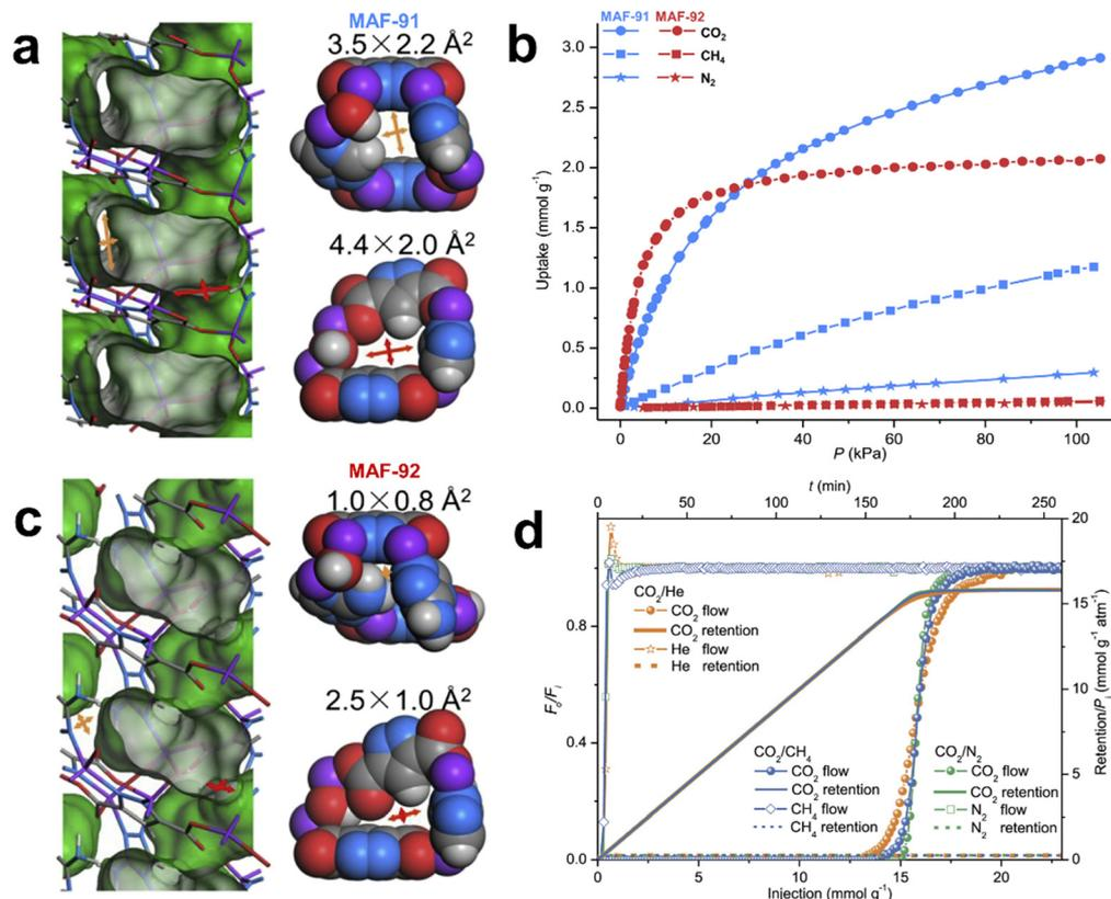
Fig. 1 (a) and (c) Crystal structures of MAF-91 and MAF-92. (b)  $\text{CO}_2$ ,  $\text{CH}_4$ , and  $\text{N}_2$  adsorption isotherms of MAF-91 and MAF-92 at 298 K. (d) Column breakthrough behaviors of MAF-92 for 10:90  $\text{CO}_2/\text{N}_2$ , 10:90  $\text{CO}_2/\text{CH}_4$  and 10:90  $\text{CO}_2/\text{He}$  mixtures. Reprinted with permission from ref. 27. Copyright 2021 Cell Press.
