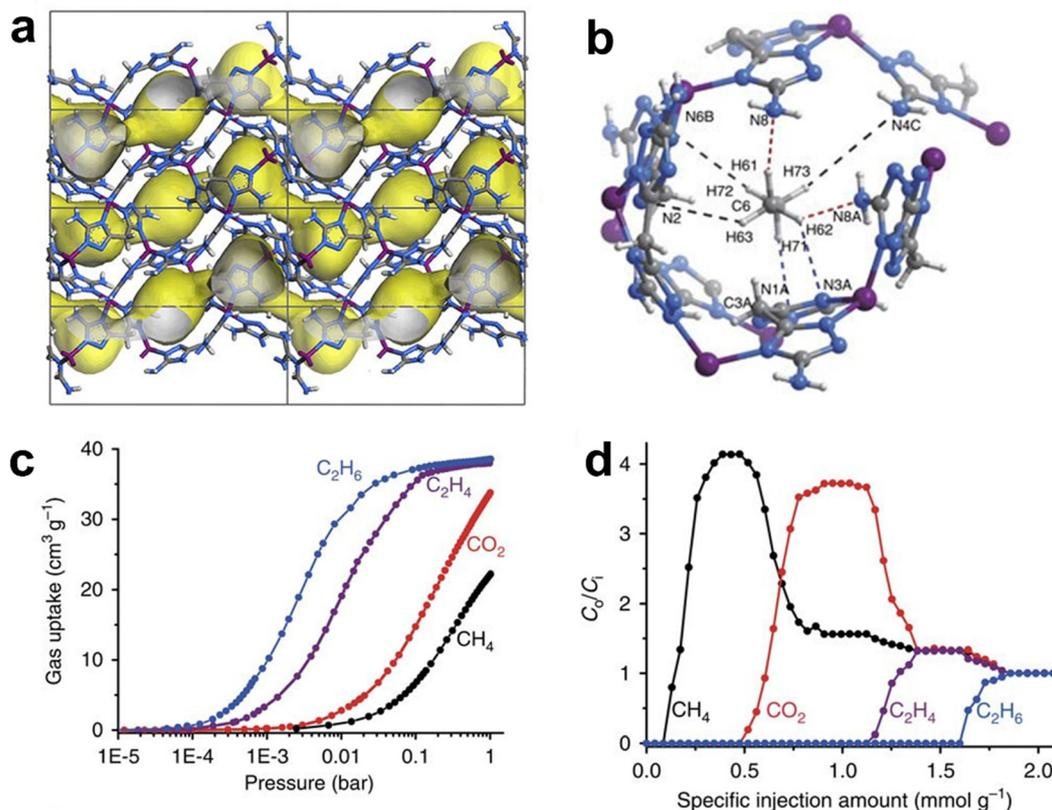
Fig. 3 (a) Crystal structure of MAF-49. (b) Preferential adsorption sites for  $C_2H_6$  in MAF-49 revealed by DFT calculations. (c) Gas adsorption isotherms for  $C_2H_6$ ,  $C_2H_4$ ,  $CO_2$  and  $CH_4$  in MAF-49 at 316 K. (d) Breakthrough curves of the  $CH_4/CO_2/C_2H_4/C_2H_6$  mixture (1 : 1 : 1 : 1 (vol)) for MAF-49 measured at 313 K and 1 bar. Reprinted with permission from ref. 59. Copyright 2018 Nature Publishing Group.
