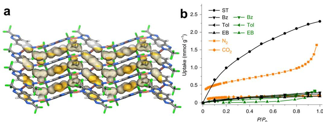
Fig. 22 (a) Crystal structure of guest-free MAF-41. (b) Adsorption isotherms of activated MAF-41 for ST (styrene, 298 K), EB (ethylbenzene, 298 K), Tol (toluene, 298 K), Bz (benzene, 298 K), N<sub>2</sub> (77 K), and CO<sub>2</sub> (195 K). Reprinted with permission from ref. 209. Copyright 2019 Nature Publishing Group.
