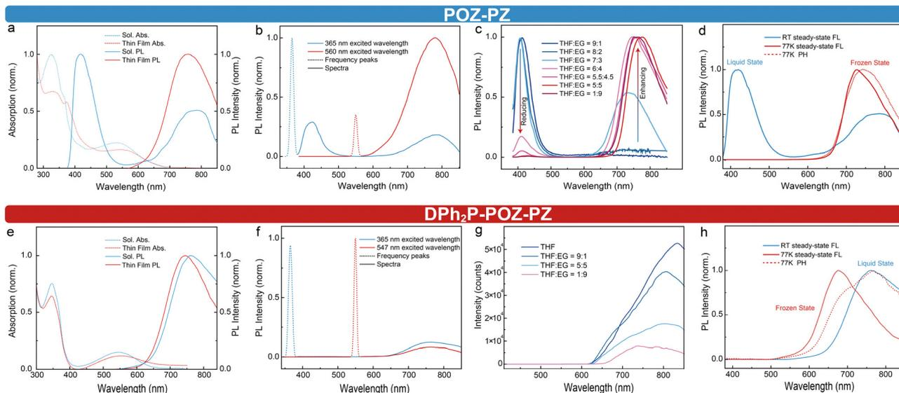
**Fig. 2** (a and e) The absorption and PL spectra in toluene solution ( $10^{-5}$  M) and pure thin film; (b and f) the PL spectra under different excitation lamps. (c and g) The viscosity-dependent spectra tested at 20 °C, volume/volume for every set; (d and h) the steady-state FL (blue line) in toluene solution ( $10^{-5}$  M) at room temperature, the phosphorescence (red dash) and steady-state FL (red line) in frozen toluene solution (identical solution with RT steady-state FL) at 77 K.
