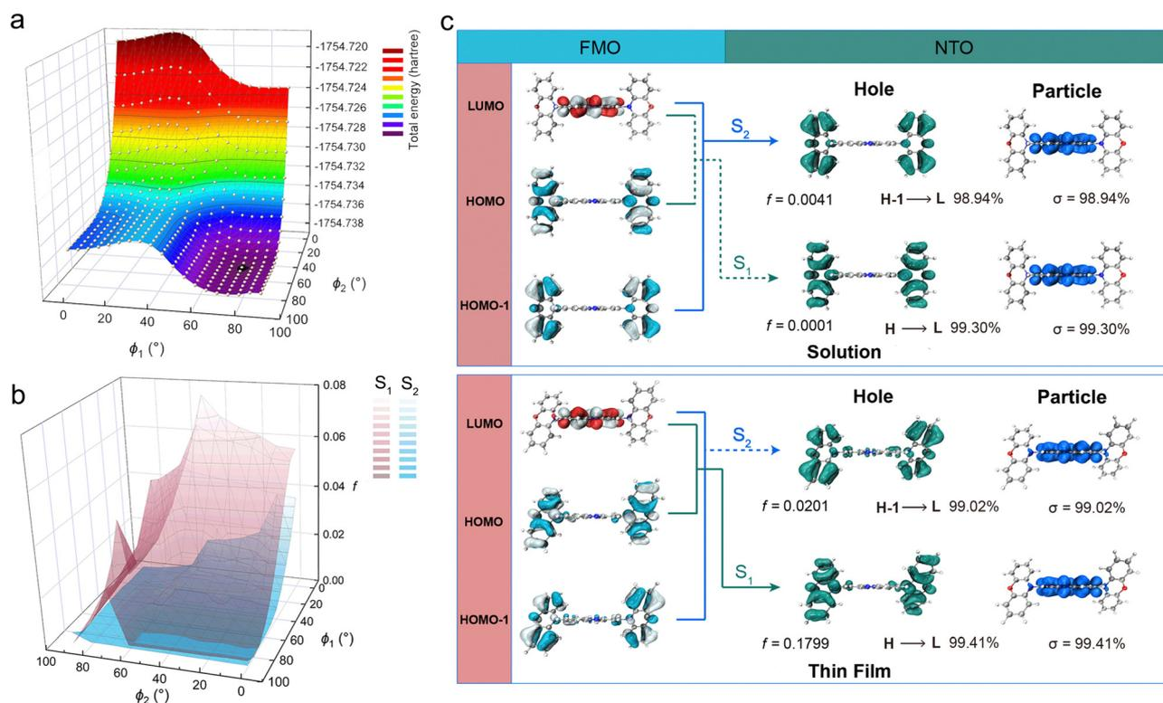
**Fig. 3** (a) The potential energy scanning of angle-dependence of POZ-PZ; (b) the oscillator strength of the excited state for angle-dependence of POZ-PZ; and (c) the surfaces of frontier molecular orbitals (sky-blue and claret-red) and natural transition orbitals (turquoise and mazarine).
