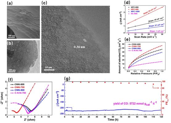
Fig. 7 (a) FESEM and (b and c) TEM images of NPC-900. (d) Dependence of charging current density differences on scan rates of the catalysts. 136 Reproduced with permission from Elsevier, copyright 2020. (e) CO<sub>2</sub> adsorption isotherms of the catalysts. (f) Nyquist plots of the catalysts. (g) Long-term stability test of CNNi-700 at -0.93 V in a flow cell. 137 Reproduced with permission from Elsevier, copyright 2021.
