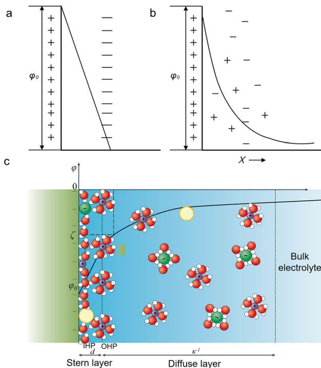
Fig. 1 Schematic description of different EDL models at a negatively charged electrode. (a) The Helmholtz model. (b) The Gouy-Chapman model. (c) The Gouy-Chapman-Stern model.<sup>40</sup> The yellow, green, purple, red, and white spheres represent neutral species, the anions, the cations, oxygen and hydrogen. Reproduced from ref. 40 with permission from the Springer Nature, copyright 2021.
