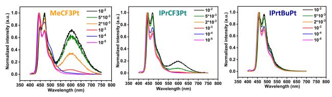
Fig. 2 Concentration-dependent PL spectra of the new Pt(II) complexes in DCM solution.
