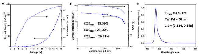
Fig. 5 (a) Current density-voltage-luminance plots, (b) current efficiency-luminance-EQE curves and (c) EL spectrum of an IPrtBuPt based hyper-OLED.
