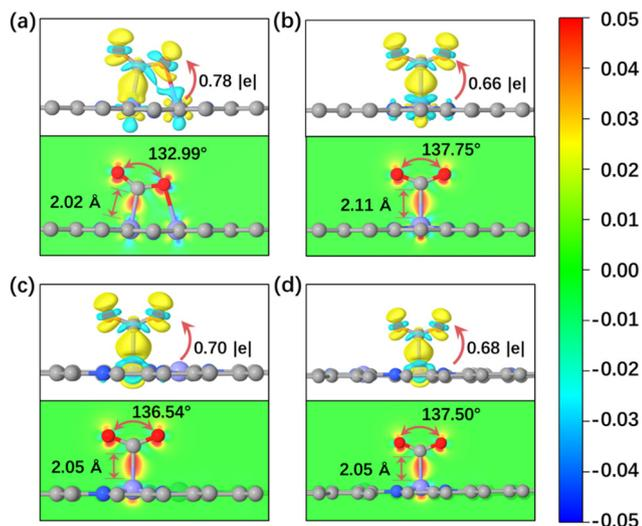
**Fig. 2** (a–d) Charge density difference and Bader charge transfer of  $\text{CO}_2$  adsorbed on  $\text{FeN}_4\text{-D}_x$  ( $x = 1, 2, 3,$  and  $4$ ) (the regions in yellow and cyan represent, respectively, electron accumulation and deletion. The isosurface levels are  $0.005 \text{ e bohr}^{-3}$ ).
