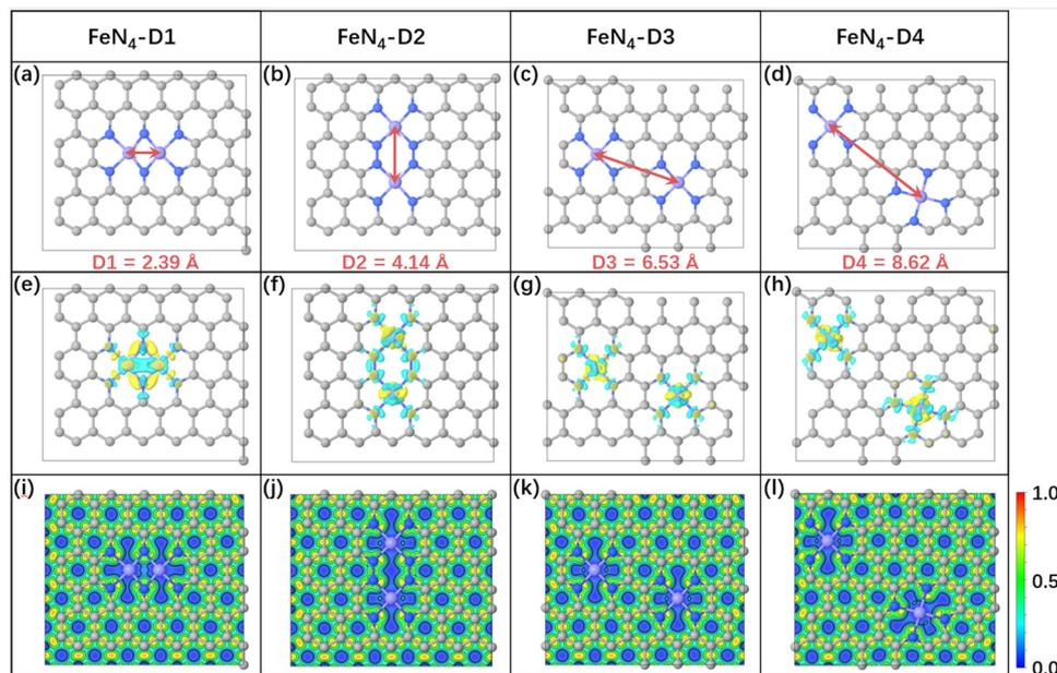
**Fig. 1** The optimized structures of four different Fe atomic pairs (a–d), charge density difference between metal atoms and nitrogen-doped carbon (e–h) (the regions in yellow and cyan represent, respectively, electron accumulation and deletion. The isosurface levels are  $0.01 \text{ e bohr}^{-3}$ ) and the corresponding electron localization function (i–l).
