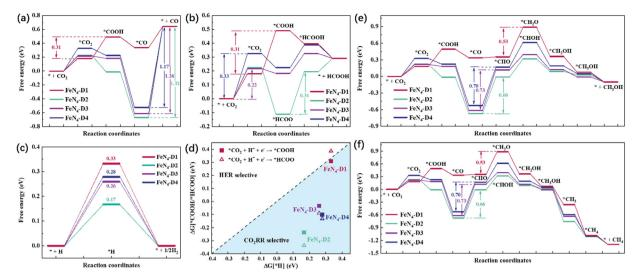
Fig. 3 Reaction free energy profile of  $CO_2$  reduction to CO (a) and HCOOH (b). HER free energy profile (c) and the comparison between the HER and  $CO_2$ RR on the four catalysts (d). Reaction free energy profile of the  $CO_2$ RR to  $CH_3$ OH (e) and  $CH_4$  (f) on  $FeN_4$ -Dx (x = 1, 2, 3, 3 and 4) structures.
