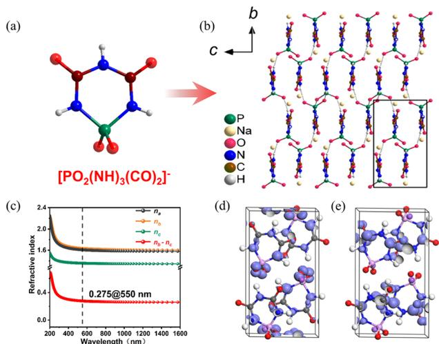
**Fig. 9** (a)  $[\text{PO}_2(\text{NH})_3(\text{CO})_2]^-$  anion. (b) Along the  $a$ -axis, the crystal structure of  $\text{NaPO}_2(\text{NH})_3(\text{CO})_2$ . (c) Theoretically calculated refractive indices and birefringence of  $\text{NaPO}_2(\text{NH})_3(\text{CO})_2$ . (d) The HOMO of  $\text{NaPO}_2(\text{NH})_3(\text{CO})_2$ . (e) The LUMO of  $\text{NaPO}_2(\text{NH})_3(\text{CO})_2$ .<sup>36</sup> Copyright 2022, Elsevier.
