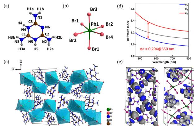
Fig. 5 (a) Crystal structure of melamine cation. (b) Crystal structure of PbBr<sub>6</sub> octahedron. (c) Viewed along the *a*-axis, the crystal structure of MLAPbBr<sub>4</sub>. (d) Theoretically calculated refractive indices and birefringence of MLAPbBr<sub>4</sub>. (e) HOMO and LUMO of MLAPbBr<sub>4</sub>.<sup>32</sup> Copyright 2022, Wiley.
