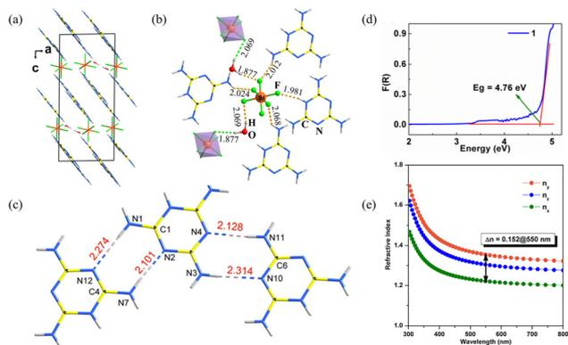
Fig. 4 (a) Structure of (C<sub>3</sub>N<sub>6</sub>H<sub>7</sub>)<sub>2</sub>SiF<sub>6</sub>·H<sub>2</sub>O viewed along the *b*-axis. (b) The coordination environment of [SiF<sub>6</sub>]<sup>2-</sup> octahedra. (c) [C<sub>3</sub>N<sub>6</sub>H<sub>7</sub>]<sub>∞</sub> chain formed by hydrogen bonds. (d) Absorption spectra. (e) Theoretically calculated refractive indices and birefringence of (C<sub>3</sub>N<sub>6</sub>H<sub>7</sub>)<sub>2</sub>SiF<sub>6</sub>·H<sub>2</sub>O.<sup>31</sup>
