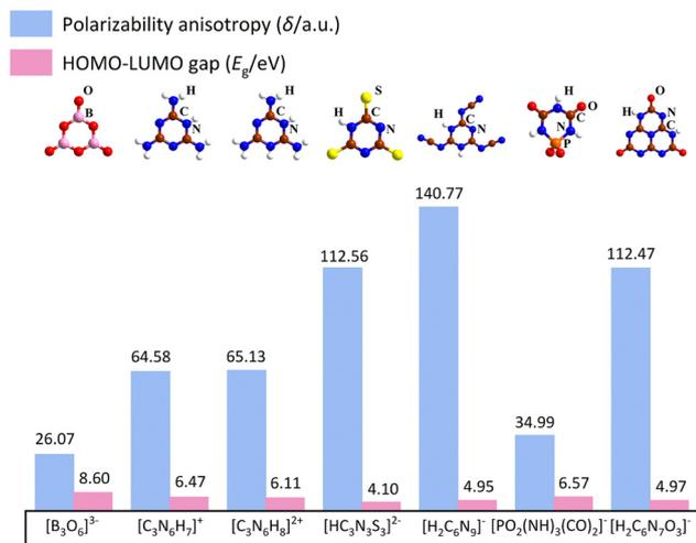
Fig. 3 Polarizability anisotropy and HOMO–LUMO gap of [B<sub>3</sub>O<sub>6</sub>]<sup>3-</sup>, [C<sub>3</sub>N<sub>6</sub>H<sub>7</sub>]<sup>+</sup>, [C<sub>3</sub>N<sub>6</sub>H<sub>8</sub>]<sup>2+</sup>, [HC<sub>3</sub>N<sub>3</sub>S<sub>3</sub>]<sup>2-</sup>, [H<sub>2</sub>C<sub>6</sub>N<sub>9</sub>]<sup>-</sup>, [PO<sub>2</sub>(NH)<sub>3</sub>(CO)<sub>2</sub>]<sup>-</sup>, [H<sub>2</sub>C<sub>6</sub>N<sub>7</sub>O<sub>3</sub>]<sup>-</sup> anion units.
