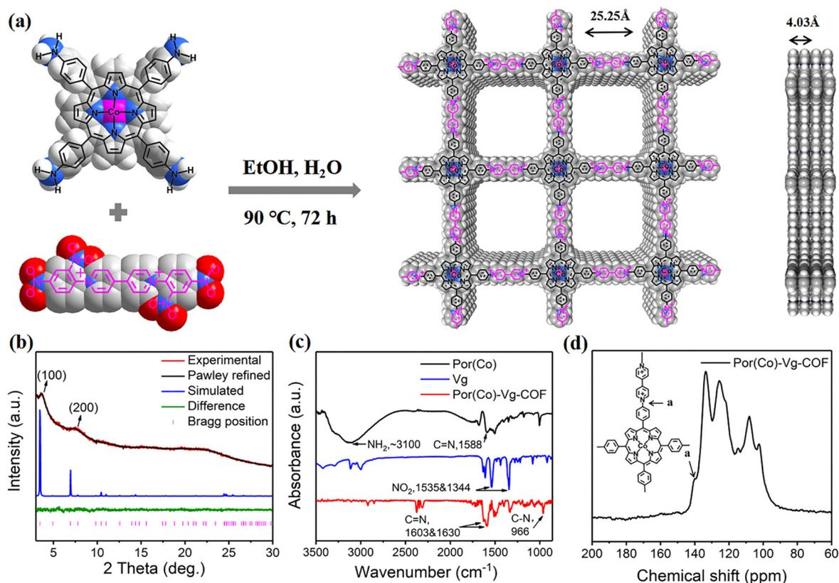
Fig. 1 (a) Illustration of the preparation of Por(Co)-Vg-COF and top and side views of their structure with  $2 \times 2$  square grids in an AA-stacking mode. (b) PXRD patterns of Por(Co)-Vg-COF. (c) FT-IR spectra of Por(Co) (black curve), Por(Co)-Vg-COF (red curve), and Vg (blue curve). (d) Solid-state  $^{13}\text{C}$  NMR spectrum of Por(Co)-Vg-COF.
