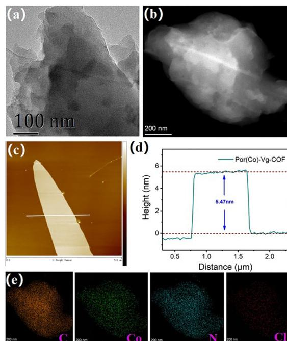
Fig. 2 (a) TEM, (b) HAADF-STEM, and (c) AFM images of Por(Co)-Vg-COF. (d) The height profile along the white line in (c). (e) The elemental mapping of C, Co, N, and Cl for Por(Co)-Vg-COF.
