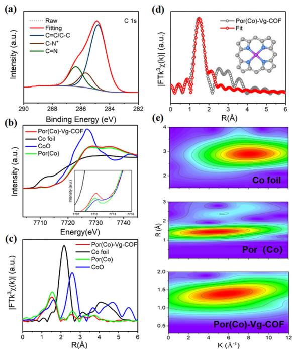
**Fig. 3** (a) High-resolution XPS spectra of C 1s for Por(Co)-Vg-COF; (b) Normalized Co K-edge XANES spectra of Por(Co)-Vg-COF, Co foil, CoO, and Por(Co); (c) Fourier-transform EXAFS spectra of Por(Co)-Vg-COF, Co foil, CoO, and Por(Co). (d) EXAFS fitting curves of Por(Co)-Vg-COF (inset: the Ni-N<sub>4</sub> architecture). (e) Wavelet transforms for the  $k^2$ -weighted EXAFS signals of different samples.
