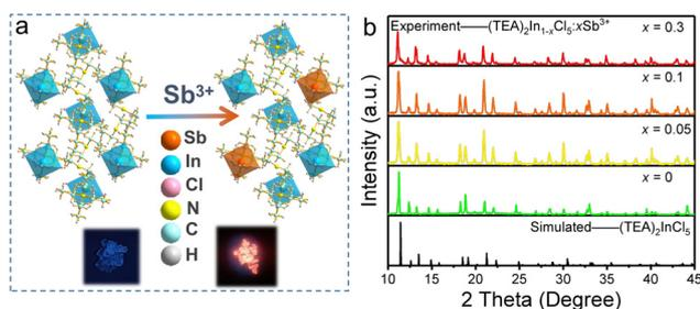
Fig. 5 (a) Doping mechanism and (b) PXRD patterns of (TEA)<sub>2</sub>In<sub>1-x</sub>Cl<sub>5</sub>:xSb<sup>3+</sup>.
