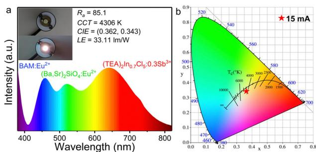
**Fig. 7** (a) PL spectra of the WLED fabricated from our  $(\text{TEA})_2\text{In}_{0.7}\text{Cl}_5 : 0.3\text{Sb}^{3+}$  and commercial blue phosphor BAM:Eu<sup>2+</sup> as well as green phosphor  $(\text{Ba,Sr})_2\text{SiO}_4 : \text{Eu}^{2+}$  on a near UV-LED chip (365 nm) at 15 mA driving current. (b) CIE chromaticity diagram of  $(\text{TEA})_2\text{In}_{0.7}\text{Cl}_5 : 0.3\text{Sb}^{3+}$  of the fabricated WLED.
