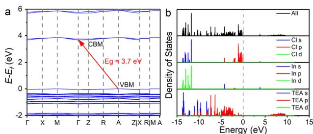
Fig. 2 (a) Calculated energy band structure. (b) The total and partial density of states of (TEA)<sub>2</sub>InCl<sub>5</sub>.
