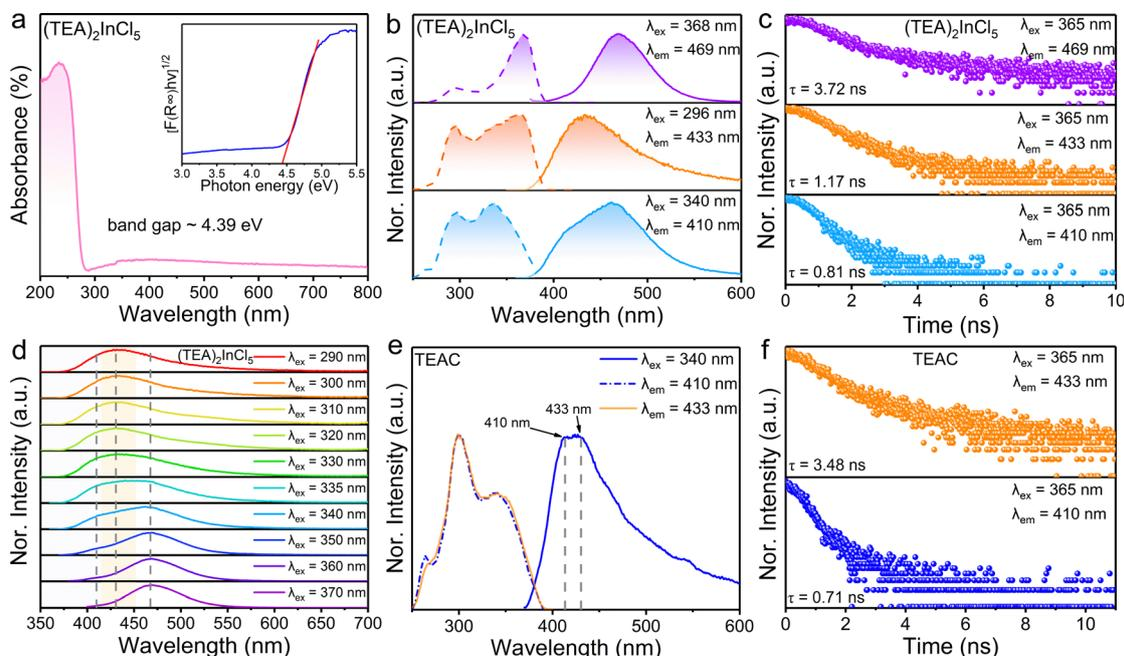
Fig. 3 (a) The absorption spectrum of (TEA)<sub>2</sub>InCl<sub>5</sub>. Inset: The Tauc plot showing the characteristics of the indirect band gap. (b) Room-temperature PLE and PL spectra of (TEA)<sub>2</sub>InCl<sub>5</sub>. (c) Room-temperature photoluminescence decay curves of (TEA)<sub>2</sub>InCl<sub>5</sub>. (d) Wavelength-dependent PL spectra of (TEA)<sub>2</sub>InCl<sub>5</sub>. (e) Room-temperature PLE and PL spectra of TEAC. (f) Room-temperature photoluminescence decay curves of TEAC.
