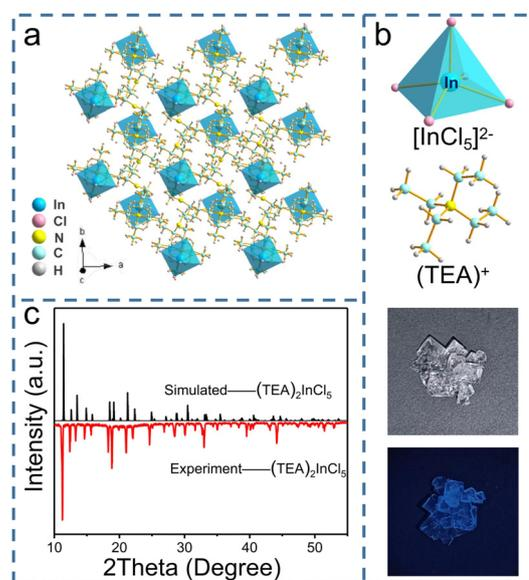
Fig. 1 (a) Crystal structure of the 0D  $(\text{TEA})_2\text{InCl}_5$ . (b) Structures of an  $[\text{InCl}_5]^{2-}$  square pyramid and organic cation  $(\text{TEA})^+$ , as well as the photographs of single crystals under natural light and 365 nm UV light. (c) Comparison of experimental and simulated PXRD patterns of  $(\text{TEA})_2\text{InCl}_5$ .
