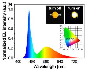
Fig. 7 Spectra, energized/unenergized photos (inset), and chromaticity coordinate chart (inset) of device 17 (a) and device 22 (b).
