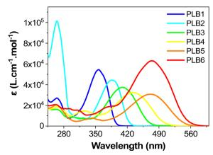
Fig. 1 The UV-vis absorbance spectra of PLB1-PLB6 in CH<sub>2</sub>Cl<sub>2</sub> solution  $(1 \times 10^{-5} \text{ mol L}^{-1})$  measured at room temperature.
