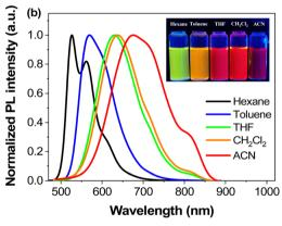
Fig. 3 Photoluminescence spectra of PLB3 (a) and PLB6 (b) in different polar solvents (1  $\times$  10<sup>-5</sup> mol L<sup>-1</sup>) and luminescence images (inset) under the irradiation of a 365 nm UV-lamp.
