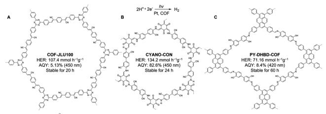
Schematics of (A) sp<sup>2</sup>c-COF-JLU100, (B) CYANO-CON, and (C) in situ Pt-PY-DHBD-COF for visible-light-driven HER.
