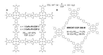
Fig. 12 Schematics of (A) CoPc-PI-COF-1 and CoPc-PI-COF-2; and (B) CNT@COF-366-R-M for CO<sub>2</sub> electroreduction in alkaline media.
