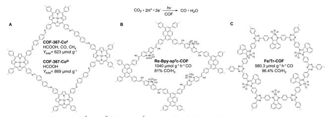
Schematics of (A) COF-367-Co<sup>II</sup> and Co<sup>III</sup>, (B) Re-Bpy-sp<sup>2</sup>c-COF, and (C) Fe/Tr-COF for CO<sub>2</sub> photoreduction under visible-light irradiation.
