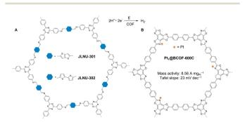
Fig. 10 Schematics of (A) JLNU-301 and -302; (B) single-atom  $Pt_1@BCOF-600C$  for electrocatalytic HER in acidic media.
