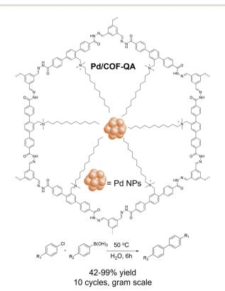
Fig. 5 Schematic of paraffin-chain quaternary ammonium salt-decorated COF supported Pd NPs for challenging chlorobenzene-based Suzuki-Miyaura coupling reaction.
