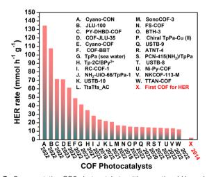
Fig. 7 Representative COF photocatalysts with exceptional H<sub>2</sub> evolution rates (>11 mmol g<sup>-1</sup> h<sup>-1</sup>) using Pt or Cu(II) as co-catalyst under visible-light irradiation. Corresponding references are summarised in Table 3.
