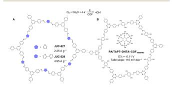
Fig. 11 Schematics of (A) JUC-527 and JUC-528, (B) PA/TAPT-DHTA- $\mathsf{COF}_{\mathsf{1000\,NH}_3}$  electrocatalytic ORR in alkaline media.
