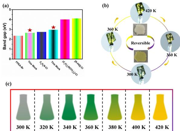
Fig. 6 (a) The band gap in this work compared with other tin-based organic-inorganic halides. (b) The temperature-induced color change in the crystal and powders of **2**. (c) A schematic of the reversible color change of **2**.
