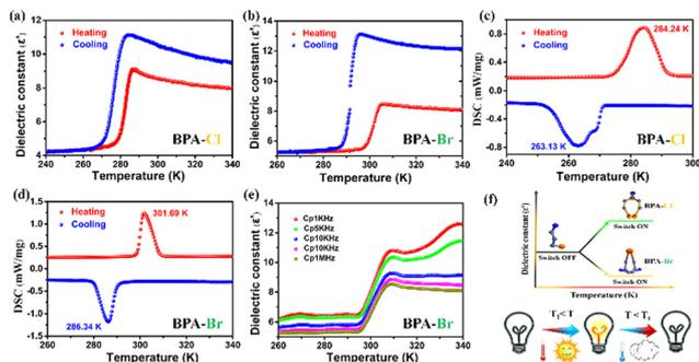
**Fig. 3** (a and b) DSC curves of **1** and **2** in heating-cooling runs. (c and d) Dielectric constant of **1** and **2**. (e) The dielectric measurement of **2** at 1 kHz, 5 kHz, 10 kHz, 100 kHz and 1 MHz upon heating. (f) A schematic diagram of the molecular switch simulation based on thermosensitive signal conversion.
