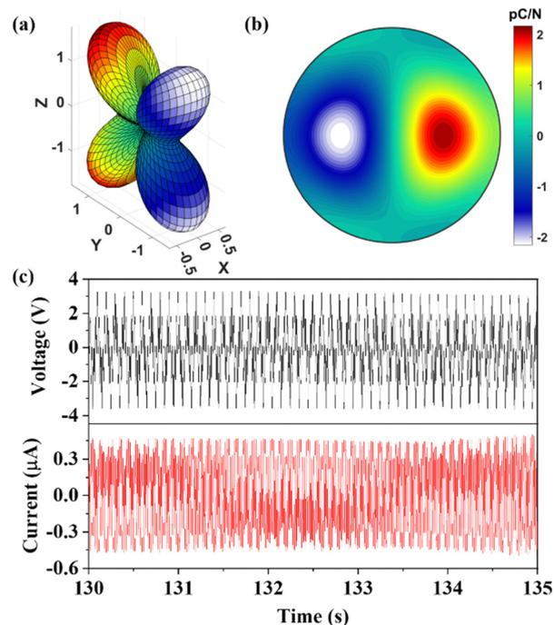
Fig. 6 (a) 3D and (b) 2D surface rendering representations of the piezoelectric strain tensors for DAP-M4. (c) Output of the open-circuit voltage ( $V_{oc}$ ) and short-circuit current ( $I_{sc}$ ) of DAP-M4/TPU film from 130 s to 135 s.
