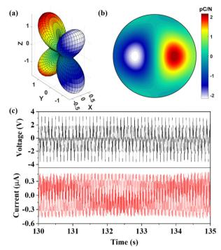
Fig. 6 (a) 3D and (b) 2D surface rendering representations of the piezoelectric strain tensors for DAP-M4. (c) Output of the open-circuit voltage  $(V_{\rm oc})$  and short-circuit current  $(I_{\rm sc})$  of DAP-M4/TPU film from 130 s to 135 s.
