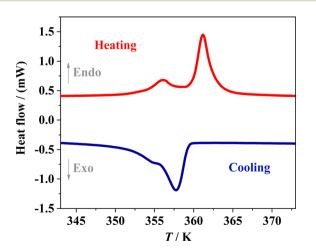
Fig. 1 DSC curves for DAP-M4 during a heating/cooling cycle.
