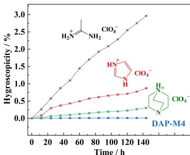
Fig. 5 Hygroscopic curves of (Ac)ClO<sub>4</sub>, (Im)ClO<sub>4</sub>, (Hdabco)(ClO<sub>4</sub>), and DAP-M4 at room temperature under 100% RH.
