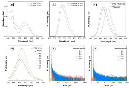
Fig. 2 (A) Absorption in toluene solution (10<sup>-5</sup> M). PL spectra (B) in toluene solution (10<sup>-5</sup> M) and (C) in the neat film and the doped film. (D) PL spectra of o-APDC-DTPA in THF/water mixtures with different water fractions (10<sup>-5</sup>M). Temperature-dependent transient PL decay spectra of (E) p-APDC-DTPA and (F) o-APDC-DTPA doped films.
