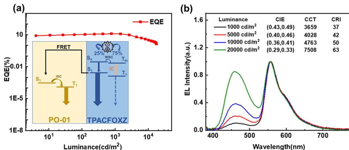
Fig. 3 (a) EQE of the device **W** and schematic diagram of the luminescence mechanism (inset), where FRET is the Förster energy transfer, IC is the internal conversion, ISC is the intersystem crossing, RISC is the reverse intersystem crossing, and T<sub>1</sub> and S<sub>1</sub> are the first triplet and singlet states, respectively. (b) EL spectra of device **W** at different luminance values.
