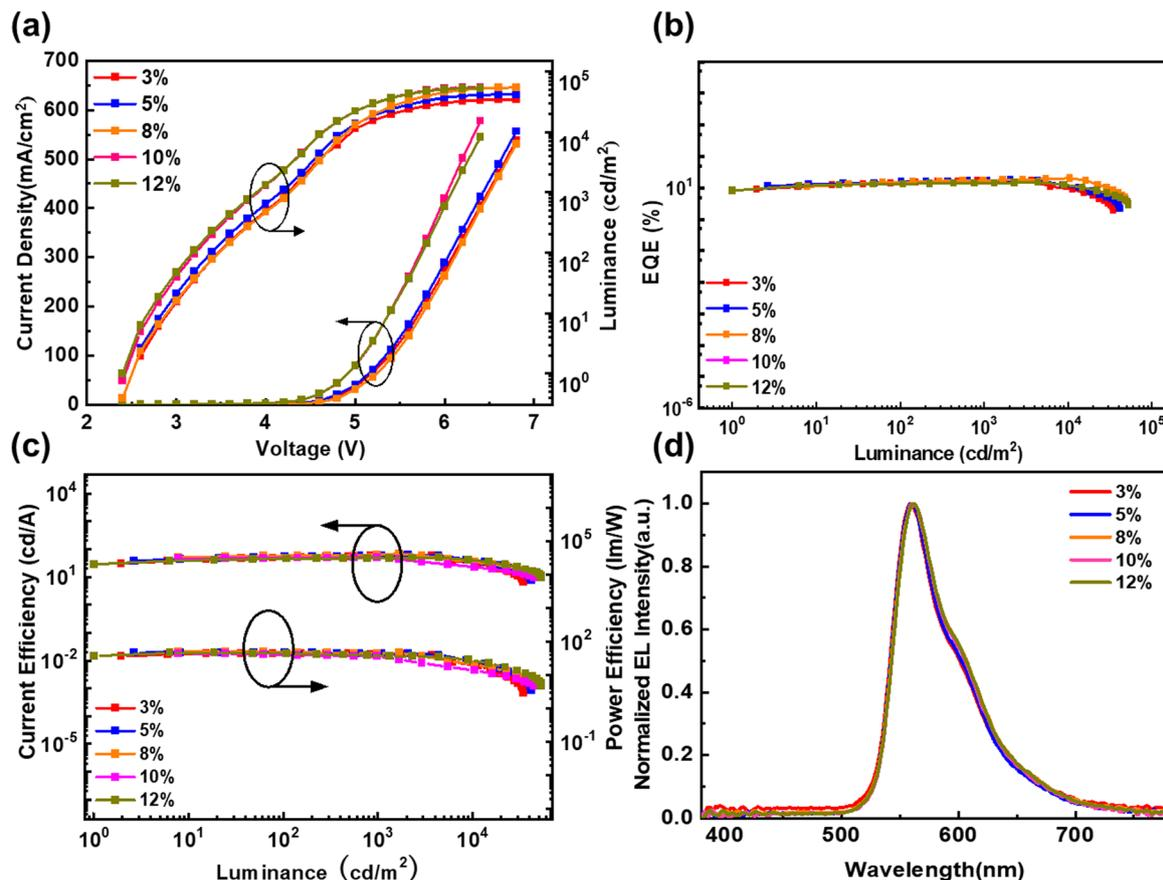
Fig. 2 EL performance of yellow OLEDs with the doping concentrations of 3%, 5%, 8%, 10%, and 12% for the PO-01 materials. (a) Current density-voltage-luminance curves. (b) EQE-luminance curves. (c) Current efficiency-luminance-power efficiency curves. (d) EL spectra at a voltage of 4 V.
