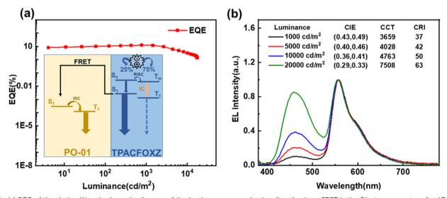
Fig. 3 (a) EQE of the device W and schematic diagram of the luminescence mechanism (inset), where FRET is the Förster energy transfer, IC is the internal conversion, ISC is the intersystem crossing, RISC is the reverse intersystem crossing, and T1 and S1 are the first triplet and singlet states, respectively. (b) EL spectra of device W at different luminance values.
