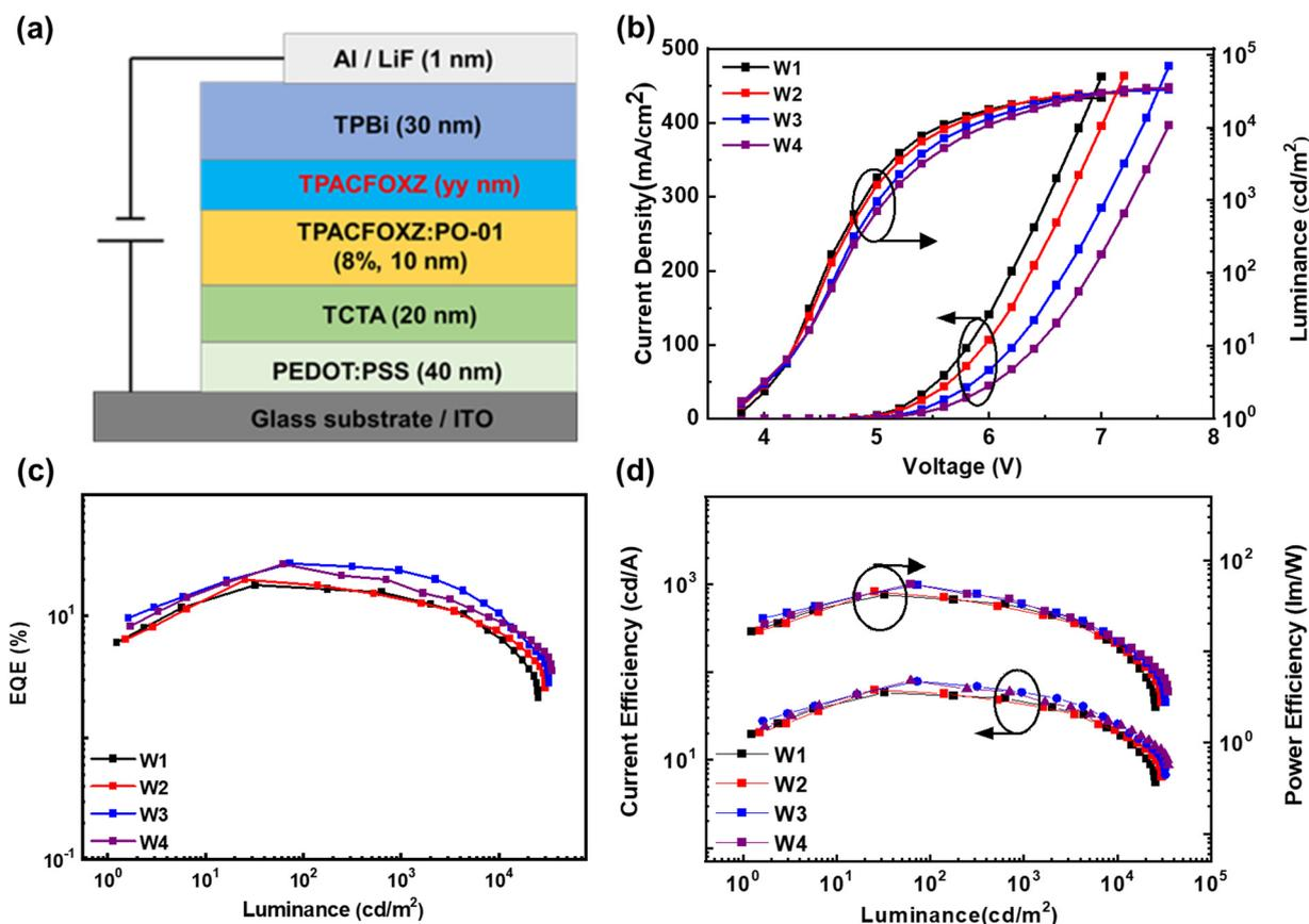
Fig. 4 (a) Device structure of YB-type WOLEDs (**W1**, **W2**, **W3**, and **W4**). (b) Current density-voltage-luminance curves. (c) EQE-luminance curves. (d) Current efficiency-luminance-power efficiency curves.
