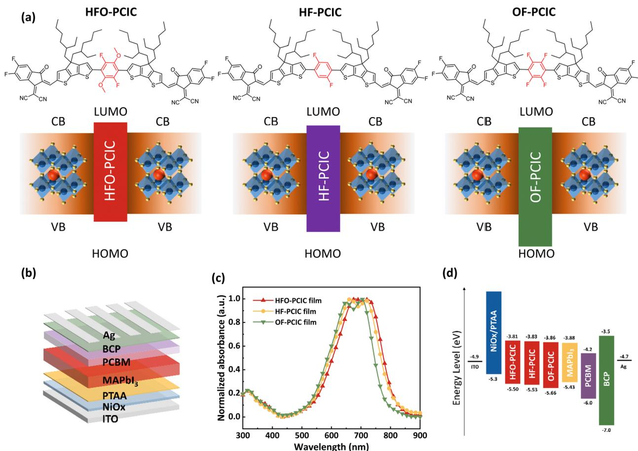
Fig. 1 (a) Chemical structures of HFO-PCIC, HF-PCIC, and OF-PCIC. (b) The schematic device structure of a typical MAPbI<sub>3</sub> PVSC device. (c) UV-vis absorption spectra of HFO-PCIC, HF-PCIC, and OF-PCIC thin films. (d) The energy level alignment of each layer.
