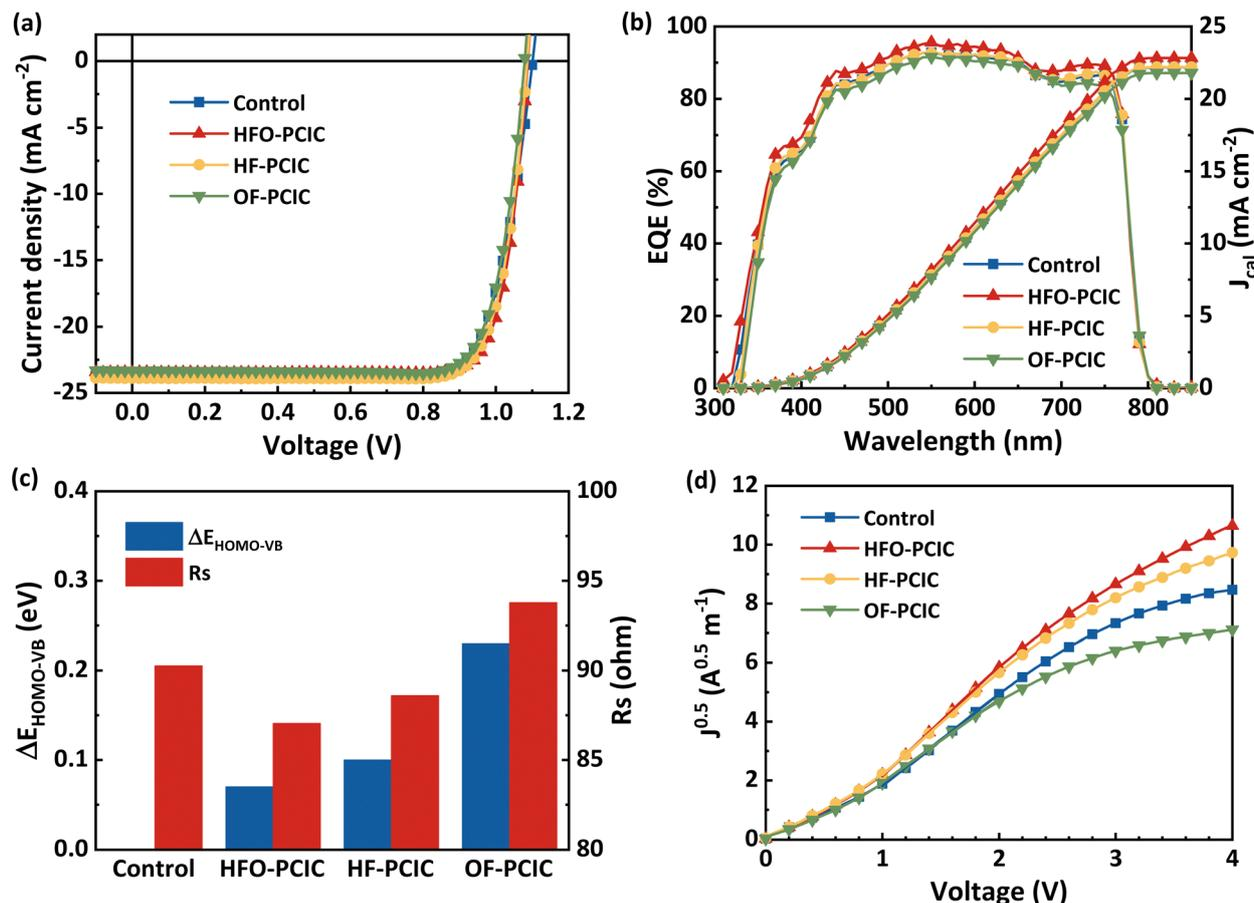
Fig. 2 (a)  $J$ - $V$  characteristics of the control and the NFA-mixed PVSCs. (b) EQE spectra and integrated  $J_{SC}$  curves of the control and the NFA-mixed PVSCs. (c) The histogram of  $\Delta E_{HOMO-VB}$  and  $R_s$ . (d)  $J^{0.5}$ - $V$  characteristics of hole-only devices, along with linear fits.
