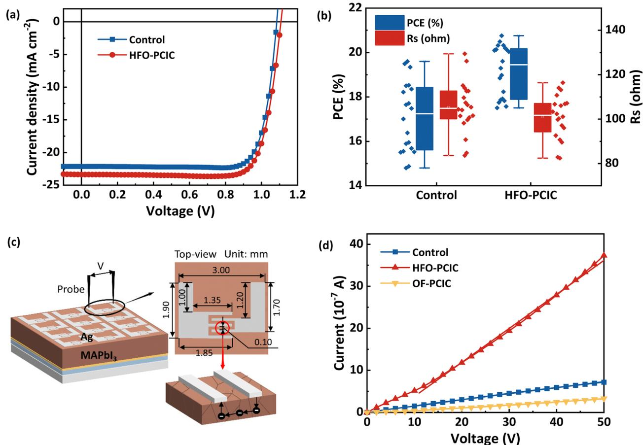
Fig. 4 (a)  $J$ - $V$  characteristics. (b) PCE and  $R_s$  distribution statistics of the PVSCs with the perovskite layer over 1500 nm. (c) The diagrammatic sketch of the test process of the horizontal charge transport. (d)  $I$ - $V$  characteristics of the PVSCs in a horizontal transmission test.
