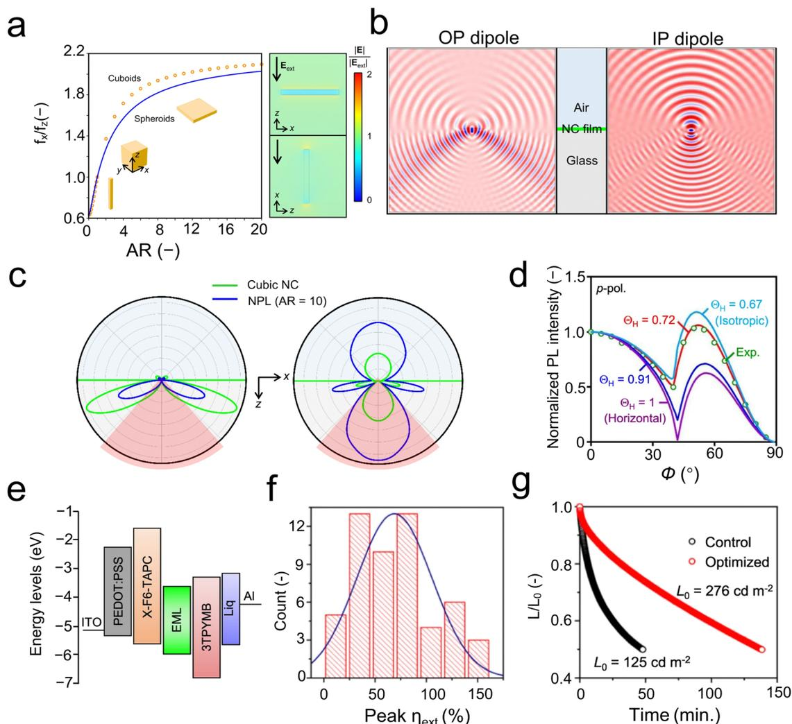
Fig. 6 (a) Calculated ratio of horizontal ( $x$ ) to vertical ( $z$ ) local field factor,  $f_x/f_z$ , as a function of the aspect ratio. Calculated electric field intensity profiles (b) and radiation patterns (c) in the  $x$ - $z$  plane for an out-of-plane (OP; left) and in-plane (IP; right). (d) Angle-dependent PL. (e) Schematic illustration of PeLEDs, and (f and g) optoelectronic properties of PeLEDs. Reproduced with Permission.<sup>79</sup> Copyright 2022, Nature Publishing Group.
