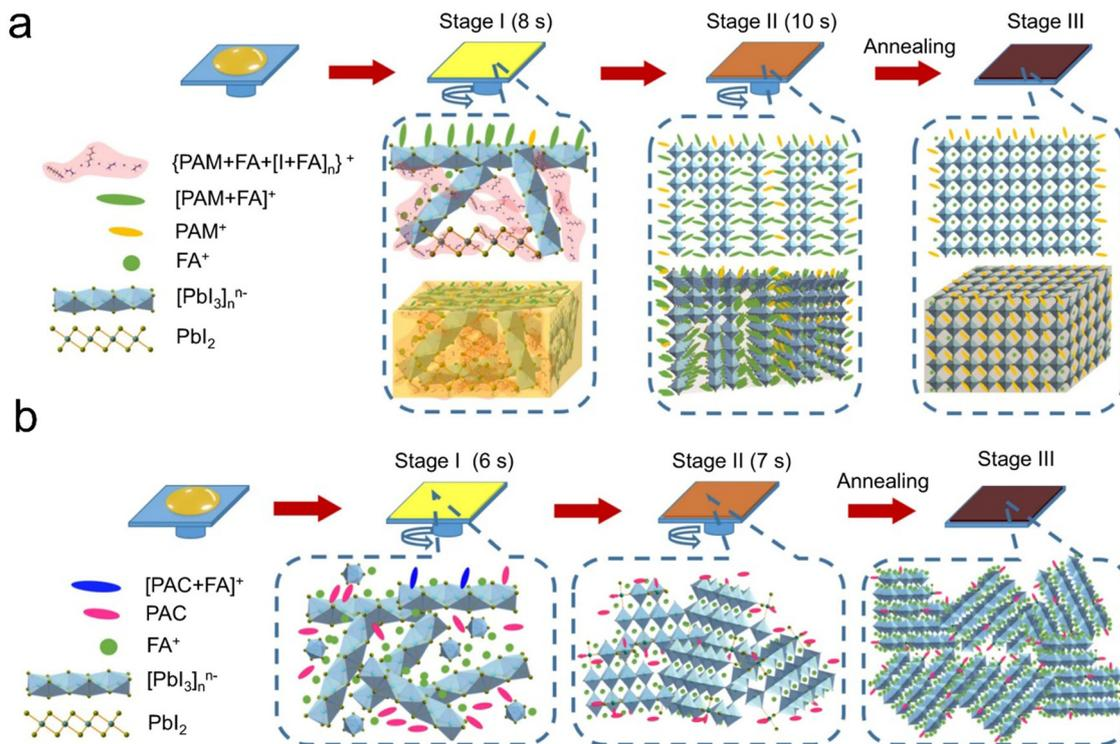
Fig. 7 (a) Pentane-1-amine-assisted oriented growth. (b) Isotropic growth with pentanoic acid additive. Reproduced with permission.<sup>107</sup> Copyright 2021, Nature Publishing Group.
