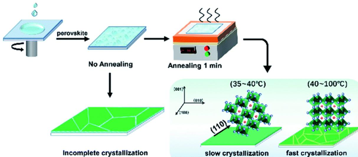
Fig. 9 Schematic illustration of the oriented growth of the perovskite with slow (35–40 °C) and fast (40–100 °C) crystallization strategy. Reproduced with permission.<sup>108</sup> Copyright 2021, Royal Society of Chemistry.
