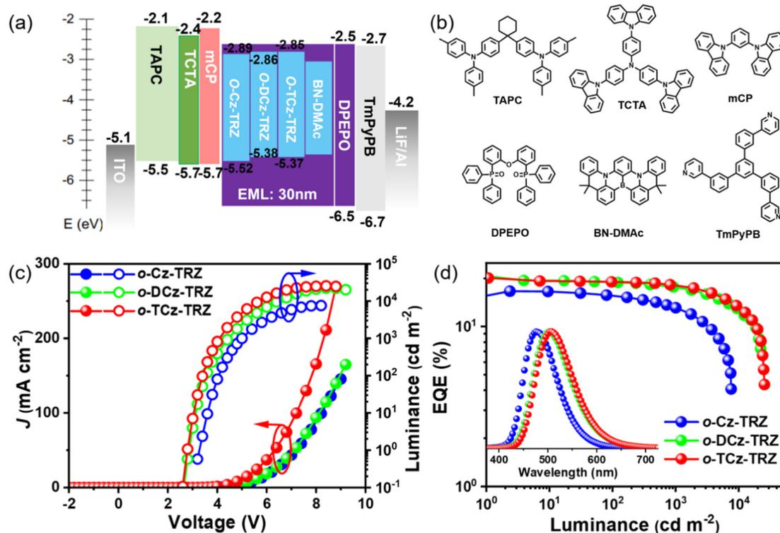
Fig. 3 (a) Device architecture and its energy level diagram. (b) Chemical structures of the corresponding materials. (c) Current density–Voltage–Luminance ( $J$ – $V$ – $L$ ) curves, (d) EQE–luminance curves and EL spectra (inset) of the devices based on *o*-Cz-TRZ, *o*-DCz-TRZ and *o*-TCz-TRZ as the emitter.
