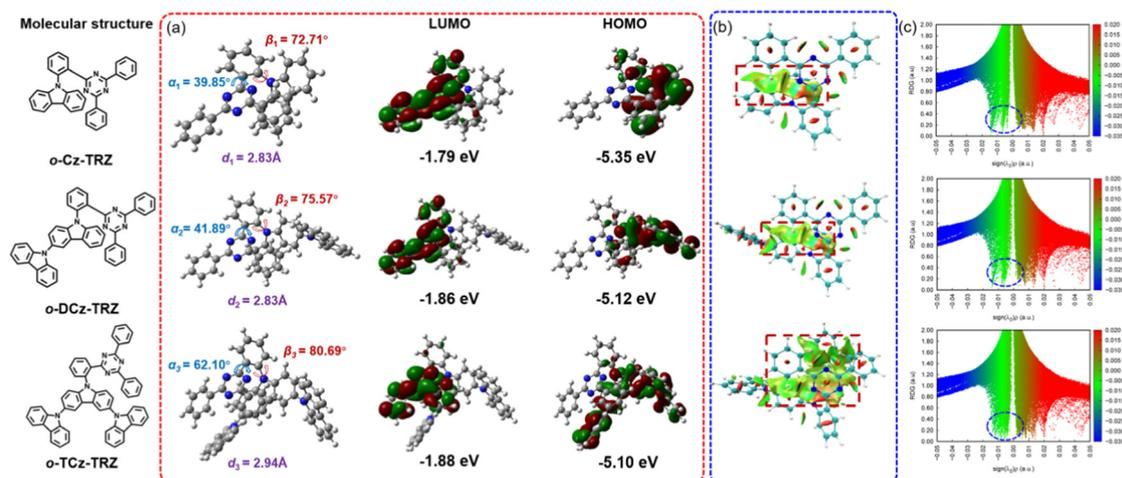
Fig. 1 Chemical structures and optimized molecular geometries of the ground states and FMO distributions and energy levels (a) simulated at the B3LYP/6-31G\*\* level. RDG isosurfaces (b) and RDG scattering diagrams (c) based on DFT simulations for *o*-Cz-TRZ, *o*-DCz-TRZ and *o*-TCz-TRZ, respectively.
