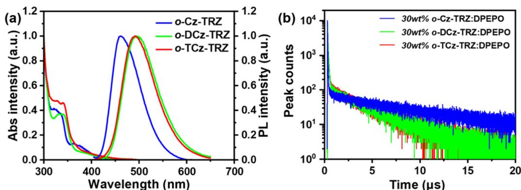
Fig. 2 (a) UV-vis absorption and PL spectra of *o*-Cz-TRZ, *o*-DCz-TRZ and *o*-TCz-TRZ in diluted toluene solution. (b) Transient PL decay curves of *o*-Cz-TRZ, *o*-DCz-TRZ and *o*-TCz-TRZ doped in DPEPO films (30 wt%).
