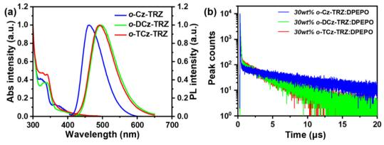
Fig. 2 (a) UV-vis absorption and PL spectra of o-Cz-TRZ, o-DCz-TRZ and o-TCz-TRZ in diluted toluene solution. (b) Transient PL decay curves of o-Cz-TRZ, o-DCz-TRZ and o-TCz-TRZ doped in DPEPO films (30 wt%).
