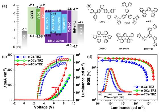
Fig. 3 (a) Device architecture and its energy level diagram. (b) Chemical structures of the corresponding materials. (c) Current density-Voltage-Luminance (J-V-L) curves, (d) EQE-luminance curves and EL spectra (inset) of the devices based on o-Cz-TRZ, o-DCz-TRZ and o-TCz-TRZ as the emitter.
