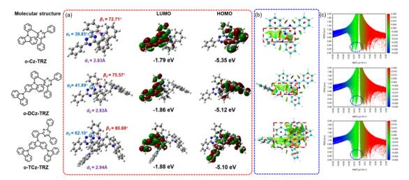
Fig. 1 Chemical structures and optimized molecular geometries of the ground states and FMO distributions and energy levels (a) simulated at the B3LYP/6-31G\*\* level. RDG isosurfaces (b) and RDG scattering diagrams (c) based on DFT simulations for o-Cz-TRZ, o-DCz-TRZ and o-TCz-TRZ, respectively.
