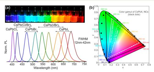
Fig. 3 (a) PL spectra and photographs of CsPbX<sub>3</sub> (X = Cl, Br, and I) MHP nanocrystals; (b) color coordinates of CsPbX<sub>3</sub> (X = Cl, Br, and I) MHP nanocrystals and the conventional LCD TV color and NTSC TV color standard. Adapted from ref. 3 with permission. Copyright 2015, American Chemical Society.
